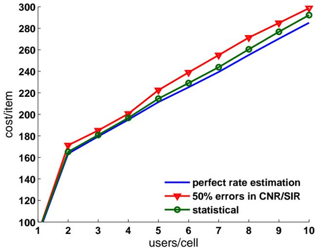
Figure 3.5: Cost comparison between optimal (perfect rate estimation) resource management, the case when errors in CNR/SIR measurement are accounted for, and the case when resource management takes the decision from statistically collected data.
