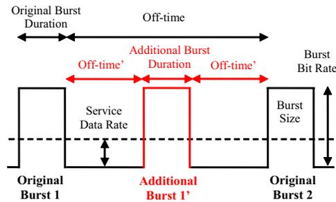
Figure 4.4: Introducing extra bursts with Raptor generated parity information in the DVB-H transmission
