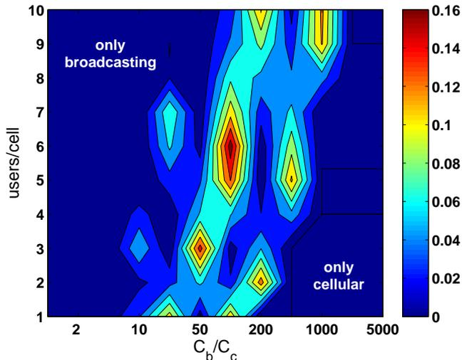
Figure 3.3: The relative cost savings obtained with 100 versus 3 broadcasting rates.
