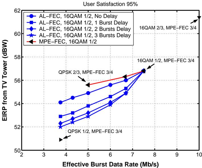
Figure 4.5: EIRP power vs. effective burst capacity
