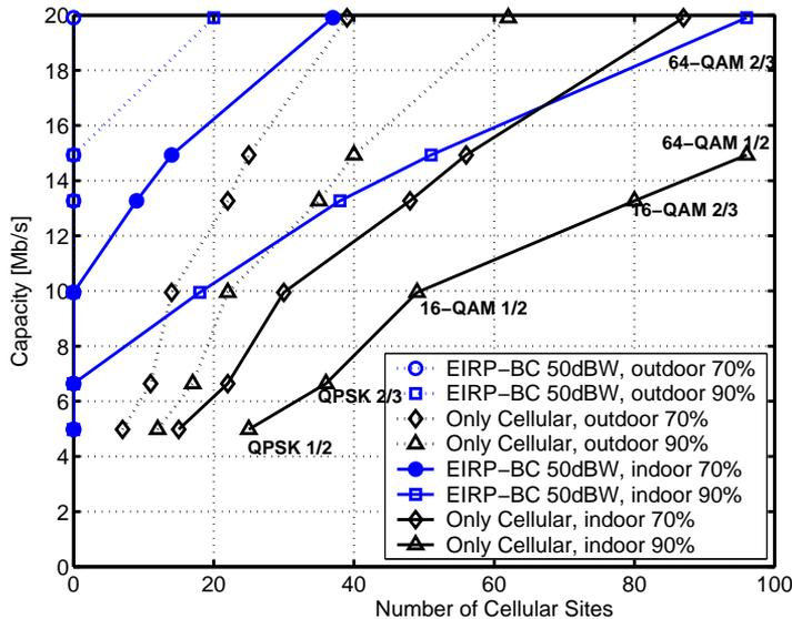
Figure 4.3: DVB-H service capacity vs. number of employed cellular sites, for different area coverage targets and EIRP values for the broadcasting tower. Service area radius is 25 km.
