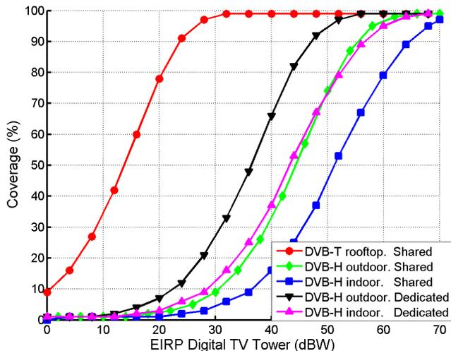
Figure 4.1: Area coverage vs. EIRP for a 150m height TV tower. Service area radius is 25 km.
