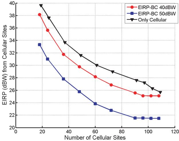
Figure 4.2: Required EIRP at a cellular site as a function of the number of sites employed. Cell radius is 2.5 km. Service area radius is 25 km (around broadcasting tower). Target coverage is 95% for indoor handheld devices.
