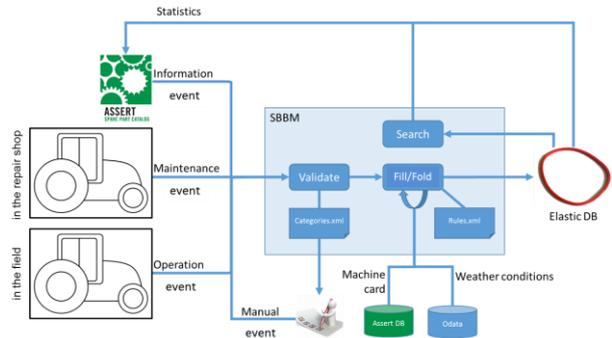
Figure 2: Data flow using an example from farming equipment (tractor)
