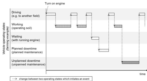
Figure 1: Exemplary vehicle operating states including changes between these states
