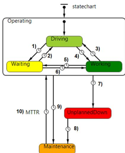
**Figure 3:** Statechart of an agent-based model for simulating industrial vehicles
