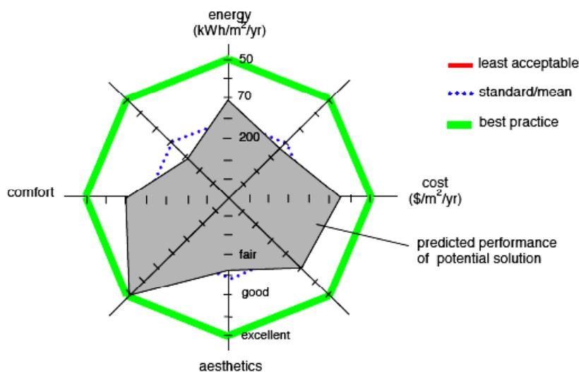
Figure 4.3. An example of a star diagram with indicated individual criteria scores and reference scores (adapted from Andresen 2000).
