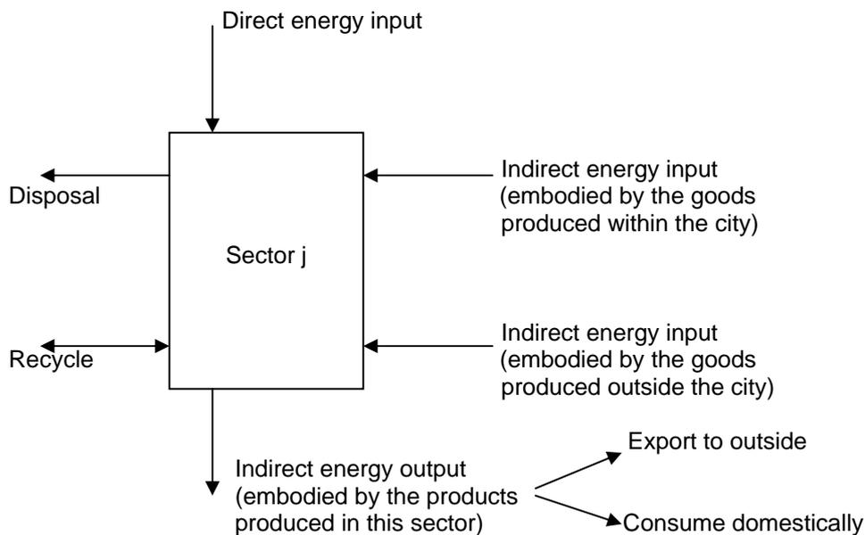
Figure 3.8. Energy balance for sector  $j$  on a city scale (adapted from Kaneko et al. 2003).
