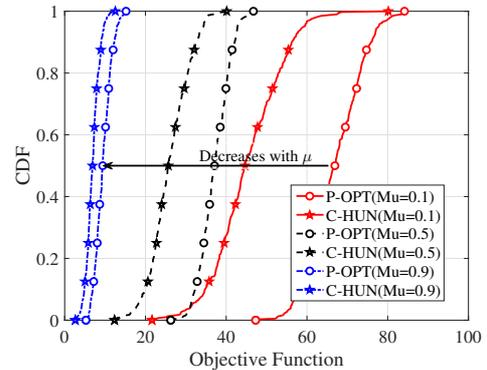
Figure 2. CDF of the objective function in Eq. (2a) for different values of  $\mu$ . We notice that the optimality gap between P-OPT and C-HUN decreases with  $\mu$ . Moreover, the objective function decreases with  $\mu$ , which is expected because of the reduction of the term with sum spectral efficiency.
