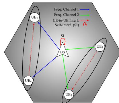
Figure 1. An example of cellular network employing FD with two UEs pairs. The BS selects pairs UE<sub>1</sub>-UE<sub>4</sub> and UE<sub>2</sub>-UE<sub>3</sub>, represented by the ellipses, and jointly schedules them for FD transmission by allocating frequency channels in the UL and DL. To mitigate the UE-to-UE interference, it is advantageous to co-schedule DL/UL users for FD transmission that are far apart, such as UE<sub>1</sub>-UE<sub>2</sub> and UE<sub>3</sub>-UE<sub>4</sub>.
