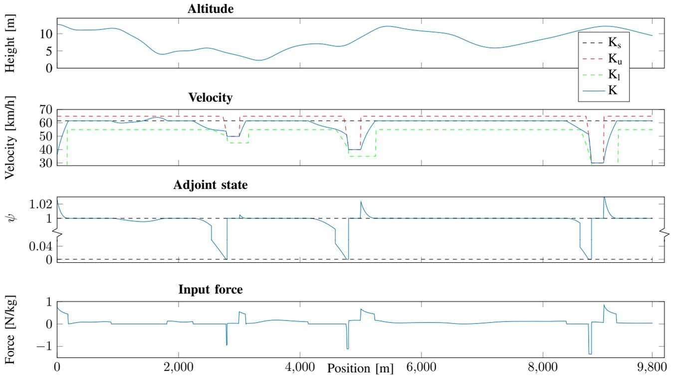
Fig. 3: Result of a simulation that uses bounding speed limits showing altitude, velocity, adjoint-state variable and tractive force. The kinetic energies are converted to the unit km/h. The plot showing the adjoint-state variable has a discontinuity for readability.
