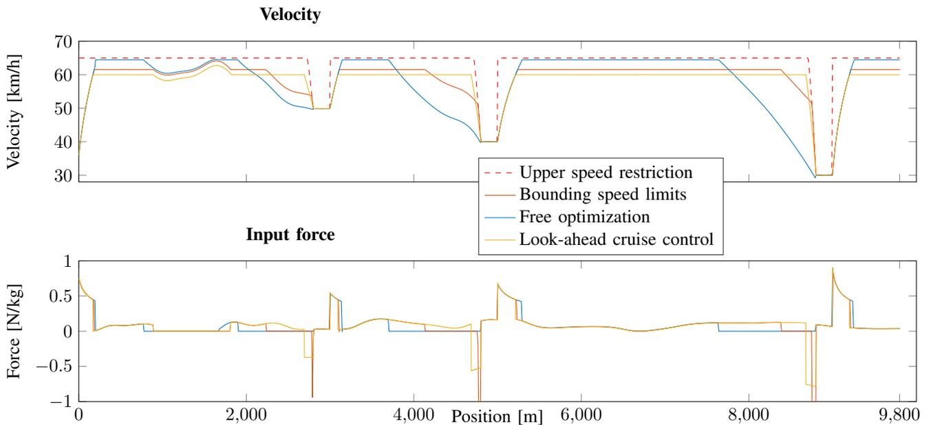
Fig. 4: Resulting velocity and tractive force from three different simulations using bounding speed limits, look-ahead cruise-control and free optimization.
