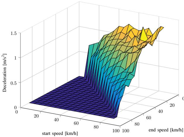
Fig. 2: Mean of rate of deceleration as a function of start and end speed.
