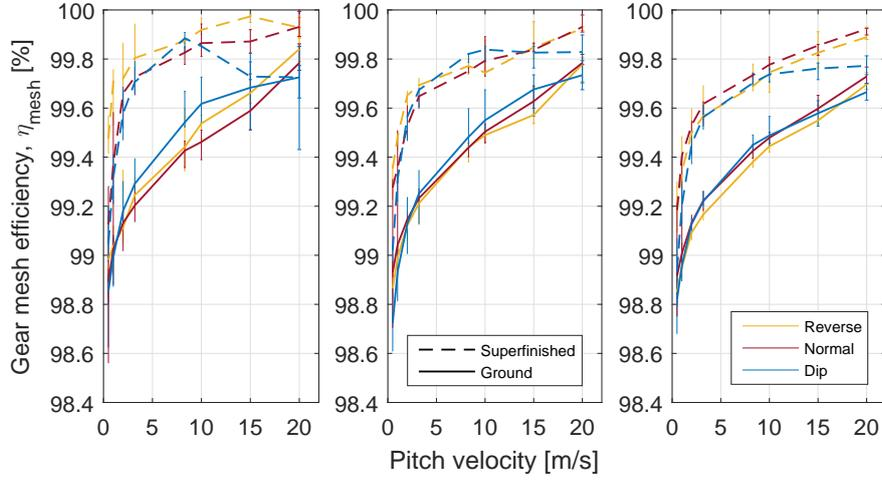
Figure 4: Gear mesh efficiency comparing ground and superfinished gears for dip and spray lubrication, run in normal and reverse direction, at contact pressures of 0.59, 0.80 and 0.96 GPa, presented from left to right. Ground gears are represented as solid lines and superfinished as dashed lines.
