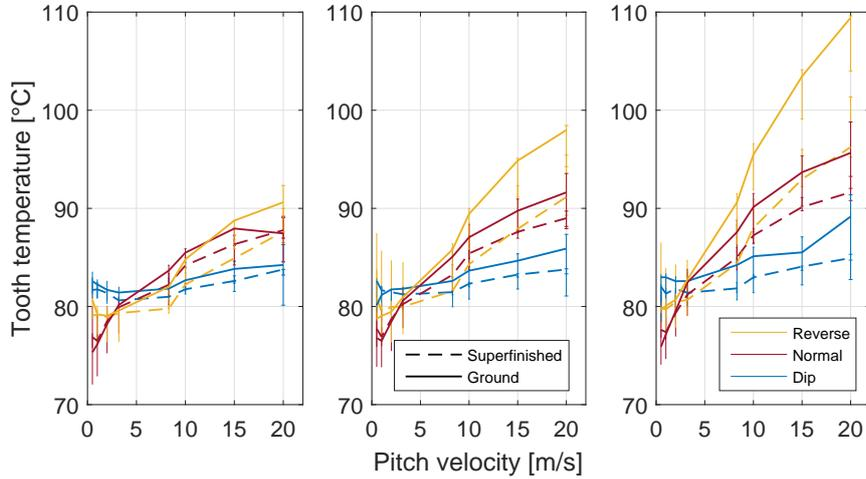
Figure 5: Measured gear tooth temperature comparing ground and superfinished gears for dip and spray lubrication, run in normal and reverse direction, at contact pressures of 0.59, 0.80 and 0.96 GPa, presented from left to right. Ground gears are represented as solid lines and superfinished as dashed lines.
