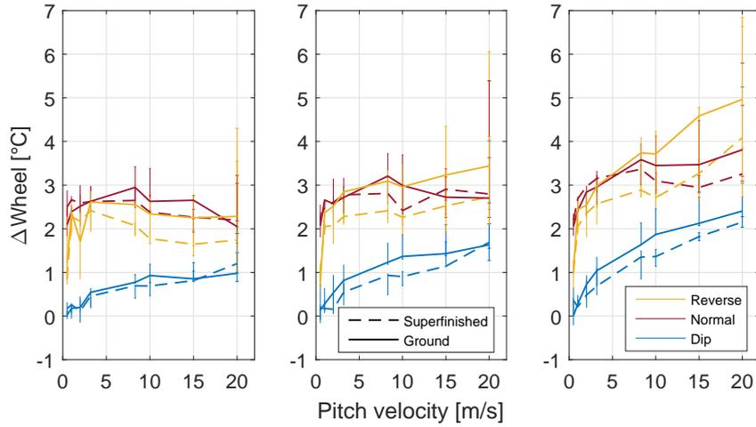
Figure 6: Measured differences between tooth and bulk temperature for ground and superfinished gears for dip and spray lubrication, run in normal and reverse direction at contact pressures of 0.59, 0.80 and 0.96 GPa, presented from left to right. Ground gears are represented as solid lines and superfinished as dashed lines.
