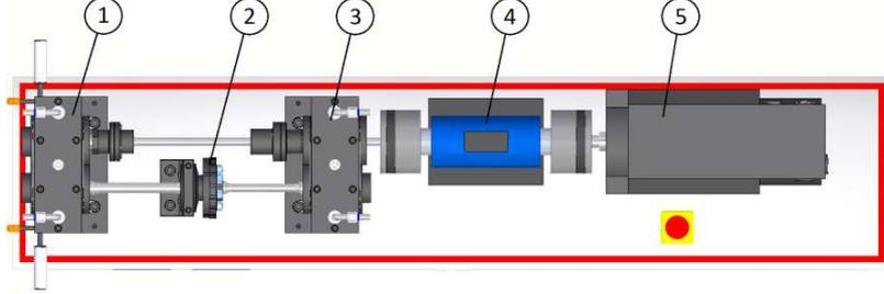
Figure 1: Top view of the FZG gear test rig, showing the test gearbox (1), load clutch (2), the slave gearbox (3), the torque and speed sensor (4) and the motor (5).
