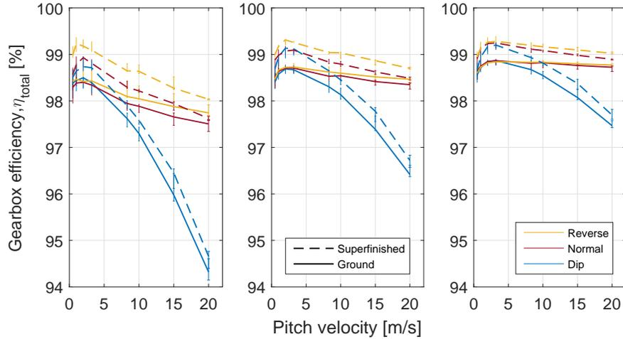
Figure 3: Gearbox total efficiency comparing ground and superfinished gears for dip and spray lubrication, run in normal and reverse direction, at contact pressures of 0.59, 0.80 and 0.96 GPa, presented from left to right. Ground gears are represented as solid lines and superfinished as dashed lines.
