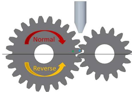
Figure 2: Sketch of the gears and the spray nozzle. In one tooth the wheel has two holes for one thermocouple each (blue and green dot). The red arrow shows when running in normal direction and the green arrow when running in reverse direction.
