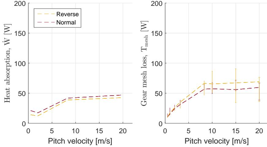
Figure 8: Heat absorbed by the lubricant is plotted on the left and mesh losses on the right for superfinished gears, at a contact pressure of 0.96 GPa.
