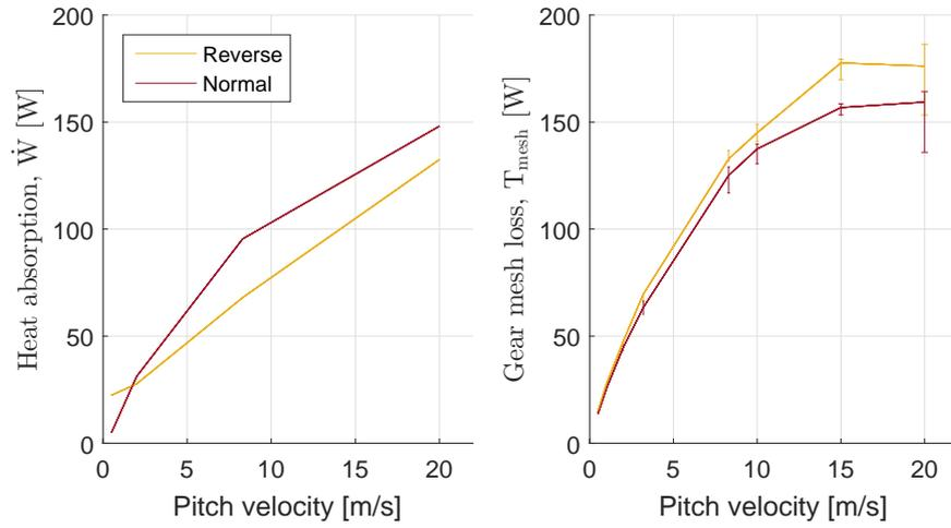
Figure 7: Heat absorbed by the lubricant is plotted on the left and mesh losses on the right for ground gears, at a contact pressure of 0.96 GPa.
