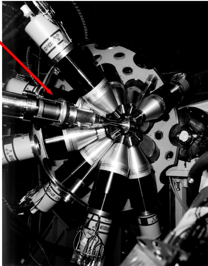
Figure 3.2: One half sphere of the Ge-array at Laboratori Nazionali di Legnaro, consisting of 40 Ge detectors, used together with the Cologne plunger, described in section 3.4.2.
