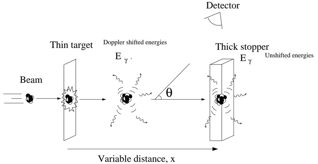
Figure 3.4: A schematic view of an RDM experiment.
