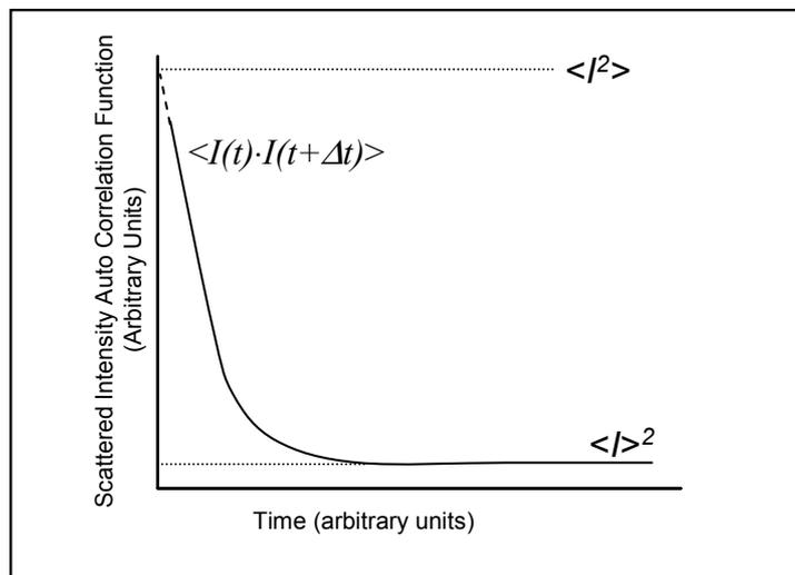
**Figure 4-3.** Time average autocorrelation function of the scattered intensity as a function of time.
