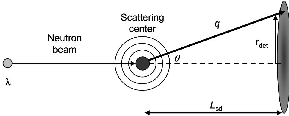
**Figure 4-5.** Schematics of the geometry of SANS experiments. See text for explanations. (Adapted from <sup>36</sup>)
