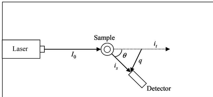
**Figure 4-1.** Schematic representation of a light scattering instrument.
