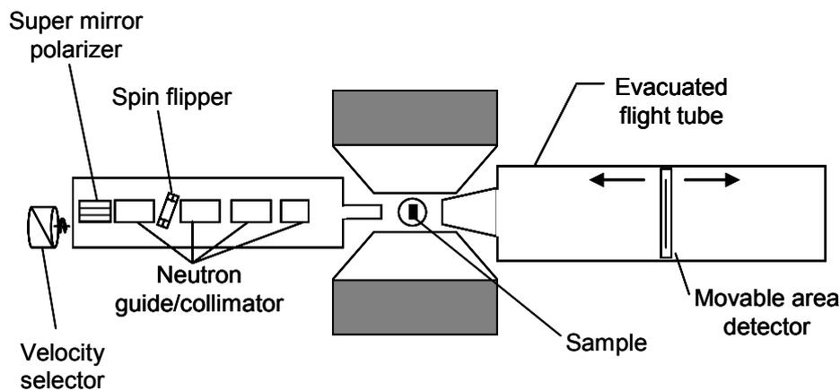
**Figure 4-4.** Schematic diagram of the fixed wavelength instrument (SANS-1) at GKSS.
