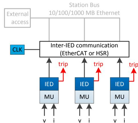
Figure 4-1 Substation architecture with combined MU and IED.
