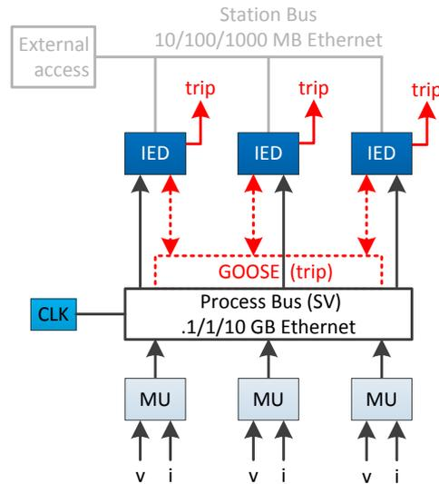
Figure 3-1 Substation architecture in IEC 61850.
