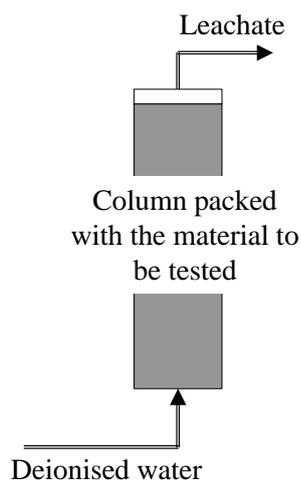
**Figure 6.** In dynamic tests, some aspects of leaching in which time is an important variable are typically addressed. One example of such a test is the upflow percolation test prEN 14405, which is under approval by CEN (European Committee for Standardisation) to become a European standard.
