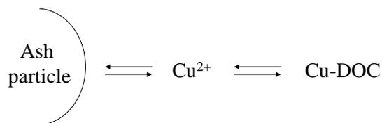
**Figure 7.** *There are several indications that Cu in the leachate from MSWI bottom ash forms complexes with DOC. Hence, the concentration of  $\text{Cu}^{2+}$  in solution is dependent on equilibrium with DOC complexes and the solid phase.*
