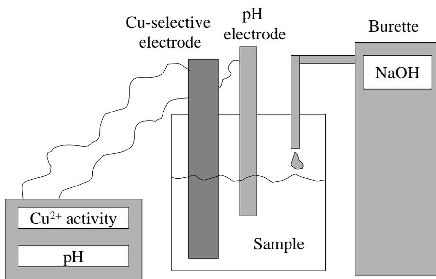
**Figure 5. Titration experiment setup for the measurement of Cu-DOC complexes at different pH values.**
