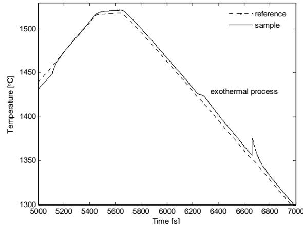
Figure 1: Temperature vs. time curve (DTA)
