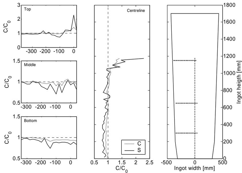
Figure 3: Segregation ratio of S and C. Sample location is shown in the right figure.
