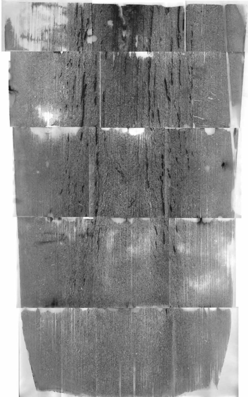
Figure 4: Sulphur print of vertical cross-section of rectangular ingot.
