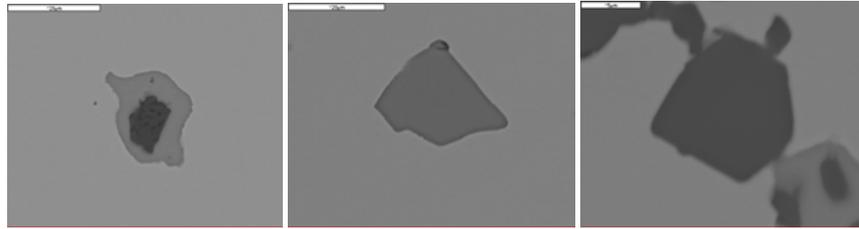
Figure 5: Duplex oxy-sulphide, pure MnS and pure  $\text{Al}_2\text{O}_3$  in high-sulphur tool steel ingot
