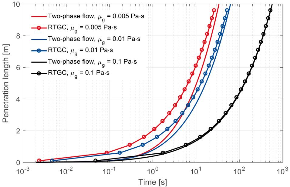
Figure 2 Penetration curves for different grout viscosity.
