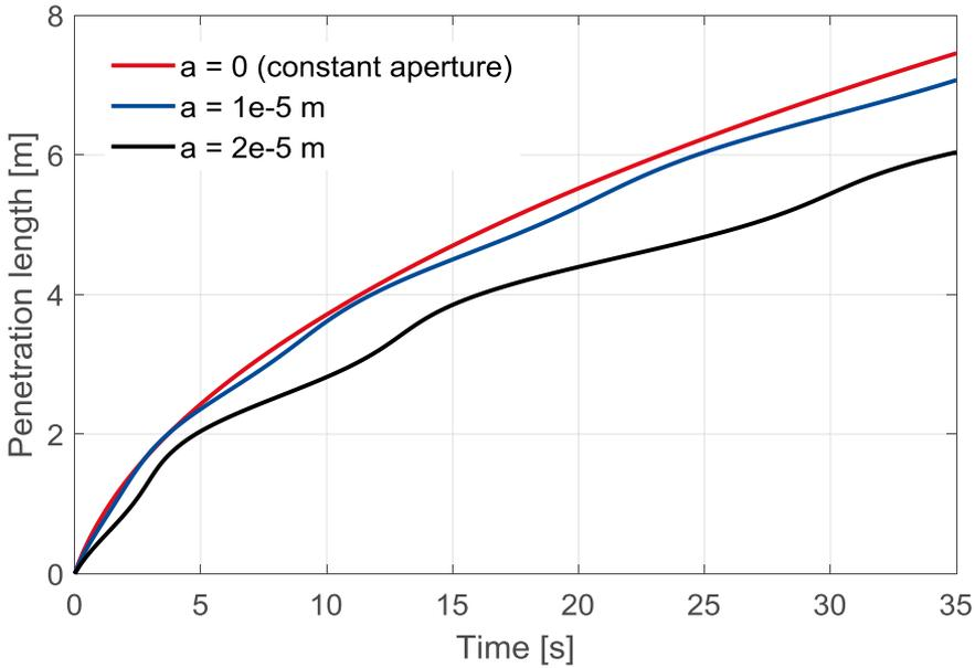
Figure 3 Penetration curves for variable fractures with different variation amplitudes.
