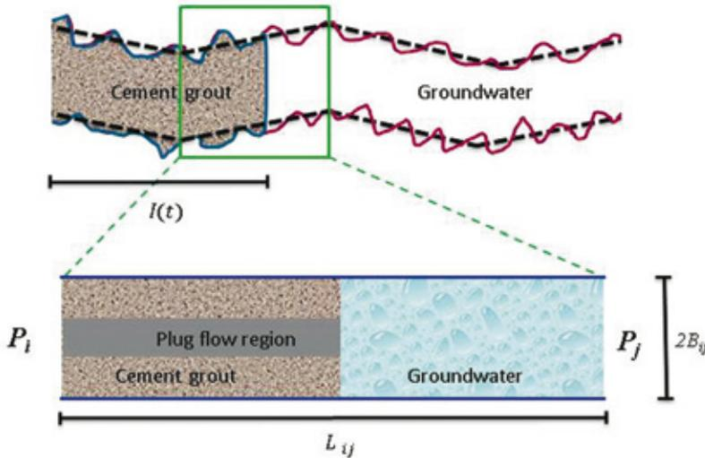
Figure 1 Illustration of cement grout penetration in a single fracture.
