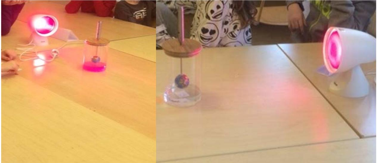
Figure 1 and 2. One lamp (the sun), one glass jar with lid (greenhouse), a thermometer fixed in a small globe (the earth). To the left, pink fluid (c-vitamin (CO<sub>2</sub>) and water), to the right only water. Two comparative experiments that were continuing at the same time.
