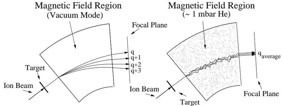
Figure 2.5: Schematic illustration of the effect of average charge collection of the recoils in a gas-filled separator. The magnetic field points perpendicular out from the page.
