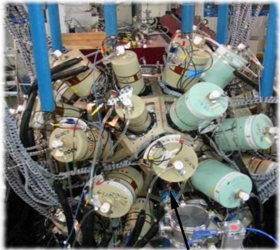
Figure 2.3: A close-up picture of the JUROGAM germanium detector array. The ion beam enters into the array from the beam line shown by the arrow at the bottom of the picture. The picture is taken from reference [9].
