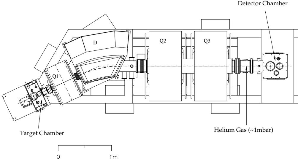
Figure 2.4: Schematic overview of the RITU recoil separator. The focusing quadrupole magnets are indicated with a Q, and D is the bending dipole magnet. The figure is taken from reference [9].
