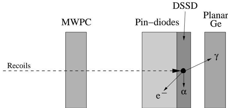
Figure 2.6: A schematic side view of the GREAT detectors. Recoils are implanted in the DSSD where subsequent charge particle ( $\alpha$  particle and proton) emission is detected. The PIN-diodes can be used for detecting electrons and escaped  $\alpha$  particles. The planar Ge-detector and the segmented clover detectors (not pictured here) are used for detection of delayed (isomeric)  $\gamma$ -ray transitions.
