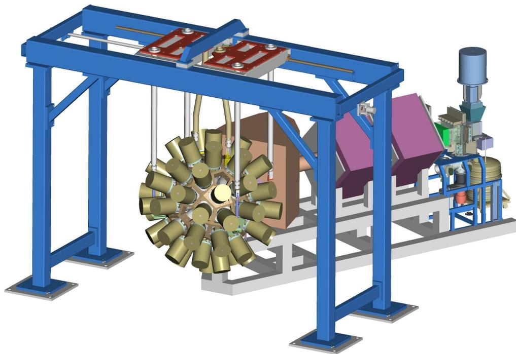
Figure 2.7: A schematic drawing of the experimental set-up. The JUROGAM Ge-array is shown in the foreground followed by the RITU recoil separator and the GREAT spectrometer situated at the RITU focal plane. The figure is taken from reference [9].
