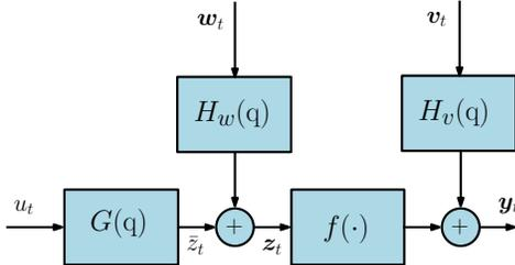
Fig. 2: Stochastic Wiener model with colored process noise
