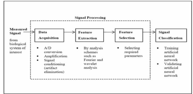
Fig. 3. Schematic of Signal Processing [42].
