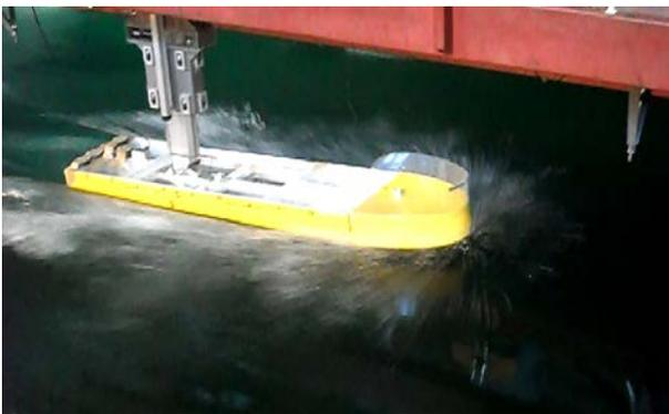
**Figure 2: UNINA model experimental set up (photo at model speed  $V = 5.75\text{m/s}$ ).**
