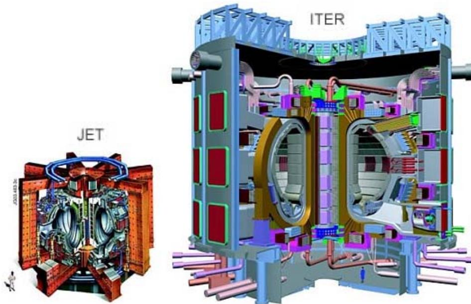
Figure 1: Cut-away diagram of the ITER device (right). Also shown is the JET device (left) for comparative purposes. Both diagrams include a 'standard man' for size perspective [18].
