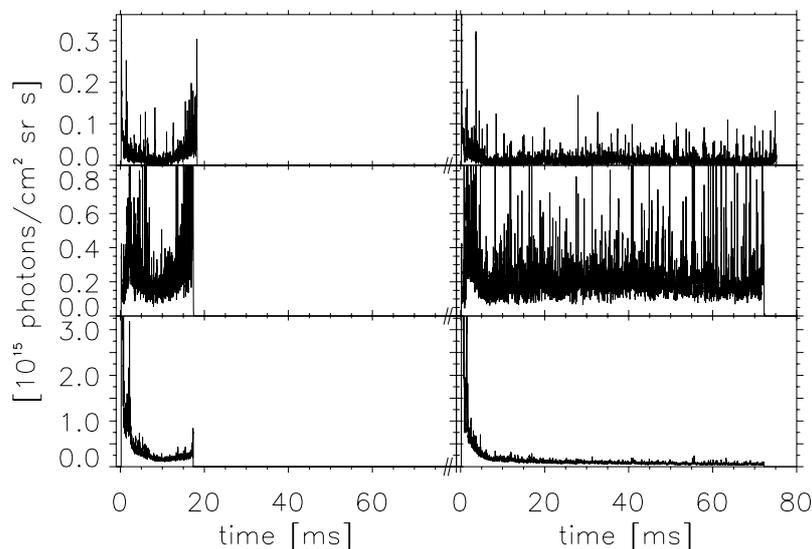
Figure 26: Typical evolution of the intensities of neutral impurities in a standard discharge (left) and in a discharge with active feedback stabilisation of the modes applied (right). The top panels show MoI (line at 319nm), the centre panels show CrI (multiplet at 359nm) and the lower panels show  $H_{\alpha}$ .
