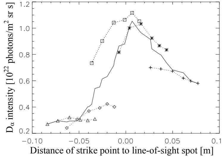
Figure 24: The  $D_\alpha$  line intensity measured during the strike point sweep where each symbol type corresponds to measurements on a different line-of-sight in the array. The solid line represents the reconstructed profile of the intensity [paper III].
