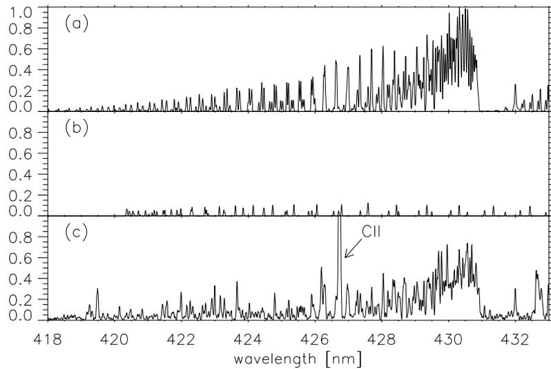
Figure 32: (a) Modelled CD Gerö band ( $A^2\Delta - X^2\Pi$ ); (b) modelled  $CD^+$  band ( $A^1\Pi - X^1\Sigma^+$ ) and (c) corresponding section of the measured spectrum from the ASDEX Upgrade divertor. The intensities of the modelled bands are normalised to lines in their respective band head regions of the experimental spectrum.
