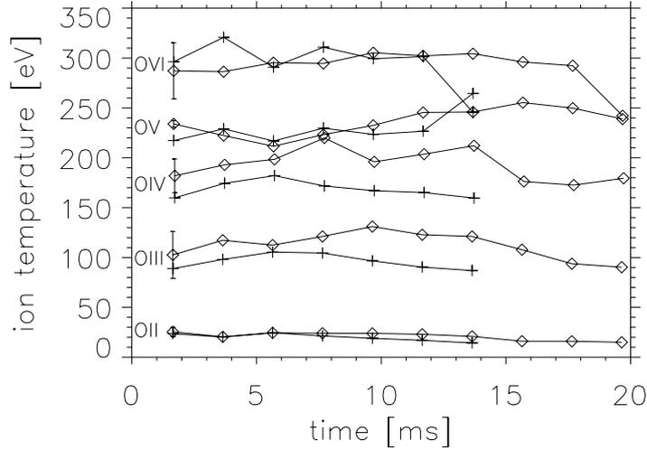
Figure 20: Time evolution of the measured the OII to OVI ion temperatures for the discharge cases with feedback mode stabilisation ( $\diamond$ ) and without (+). The average error bars for each ion are indicated on the first point of each curve with feedback.
