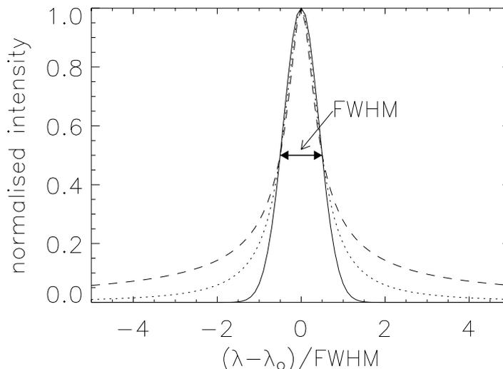
Figure 5: Line shape for Gaussian (—), Lorentzian (····) and general line shape with maximum tails (---) with equal full width at half maximum (FWHM) and peak intensity, calculated from [25].
