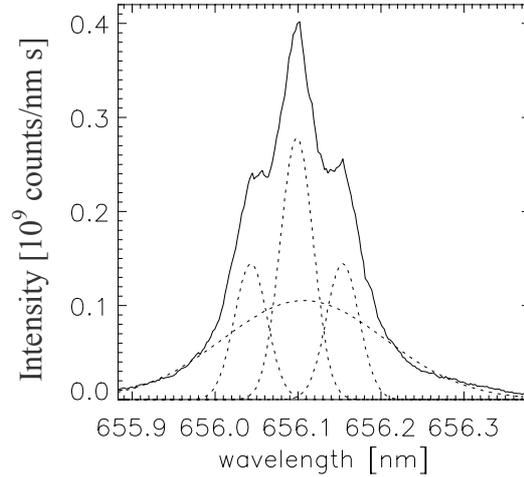
Figure 7: Zeeman split  $D_\alpha$  line measured in the ASDEX Upgrade outer divertor (full line) with fitted components (dotted curves) [paper III]. The broad component is included to better match the wings.
