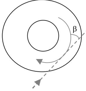
Figure 17: The angle  $\beta$  between the toroidal rotation (curved arrow) and the mid-plane toroidal line-of-sight (dashed arrow).
