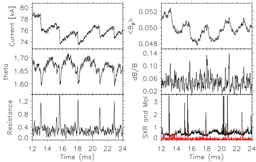
*Figure 33: The periodic large fluctuations observed in plasma current ( $I_p$ ), theta ( $\theta$ ), resistance, average toroidal field  $\langle B_\phi \rangle$ , total magnetic fluctuation level  $dB/B$  and in last panel SXR intensity (black) and Mol intensity (lighter) [paper V].*
