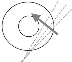
*Figure 11: An array of lines-of-sight intersecting a neutral beam (thick arrow) can be used for spatial profiling through localised emission where the plasma interacts with the beam.*
