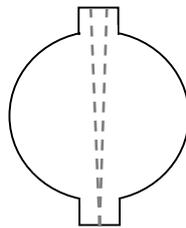
Figure 14: The line-of-sight is not a one-dimensional line but instead consists of a cone that spreads out. The angle shown here is exaggerated compared to that of the fibre used for the EXTRAP T2R rotation measurements.
