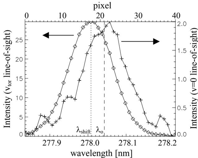
Figure 6: Typical OV line (278nm) as measured on the central poloidal line-of-sight, the zero-velocity position, (right axis and curve with +) and on the mid-plane toroidal line-of-sight (left axis and curve with  $\diamond$ ).
