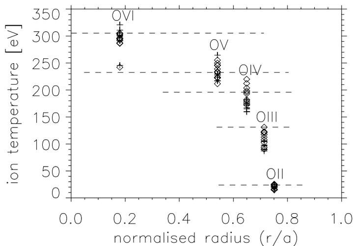
Figure 21: The measured  $T_i$  of figure 20 as a function of radial position of the ions. The points ( $\diamond$  with feedback and + without) are plotted at the radial position of the peak in the respective ion emissivity profiles and the horizontal dashed lines represent the FWHM of these curves.
