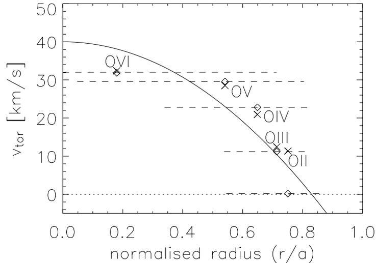
Figure 19: Reconstruction from paper IV of the radial profile of the toroidal ion velocity  $v_{tor}(r)$  (solid line), which results in the modelled (x) ion velocities  $v_i$ . The experimental velocities (◇) at a single point are shown for comparison. The horizontal dashed lines indicate the FWHM of the emission curves whilst the points are plotted at the radii of their respective emissivity peaks.
