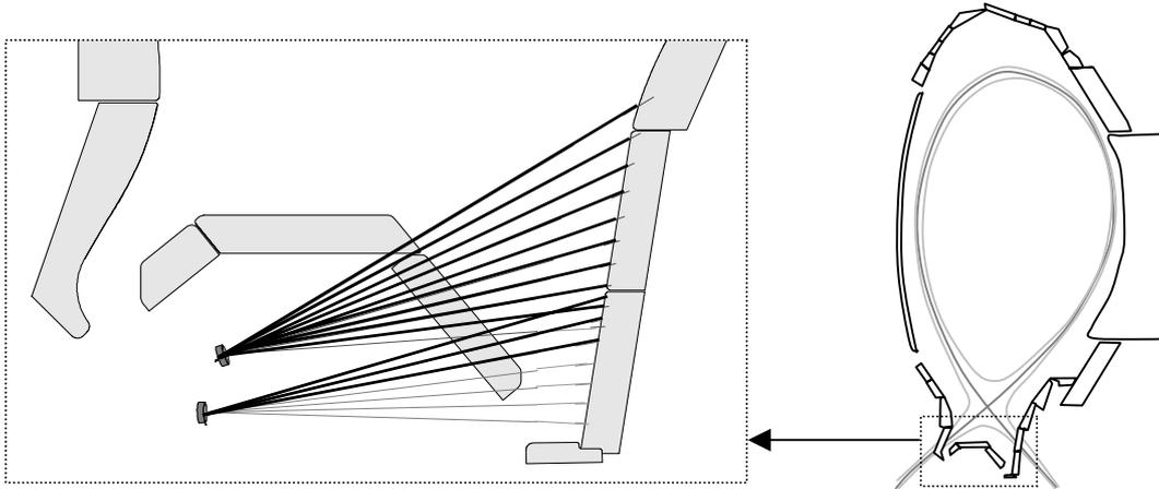
*Figure 23: Cross-section of ASDEX Upgrade with enlargement of the divertor region showing the outer divertor line-of-sight array, the darker lines-of-sight were those used in the experiments of paper III.*
