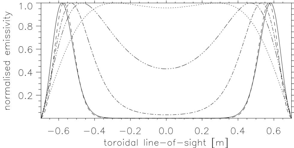
Figure 18: Normalised emissivity profiles along the mid-plane toroidal line-of-sight for the ions OII (—), OIII (---), OIV (- · -), OV (- - -) and OVI (····). Converted from radial profiles measured with the five-channel spectrometer described in papers VIII and XI.
