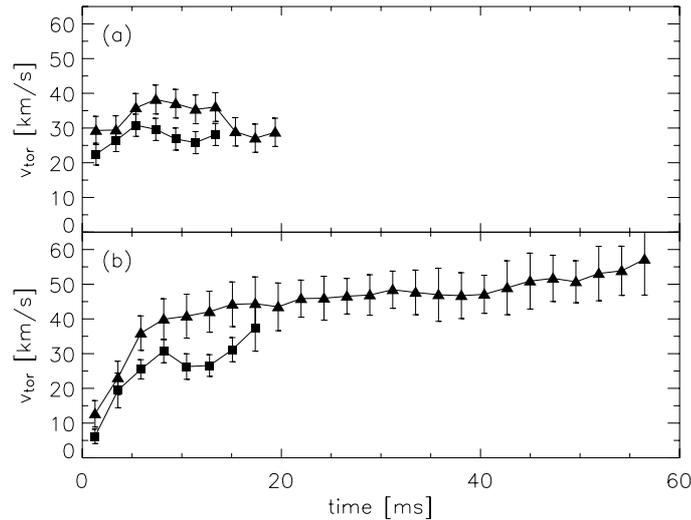
Figure 26: Evolution of the OV toroidal rotation velocity for discharges with (▲) and without (■) active feedback stabilisation in the cases (a) paper IV and (b) paper VI.
