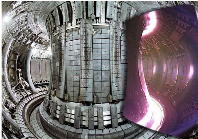
*Figure 4: The inside of the JET tokamak (2005): (left) without plasma and (right) with plasma (in infra-red) [18]. The D-shaped plasma cross-section and divertor structure at the bottom of the tokamak, where the light is most intense, can be clearly seen.*
