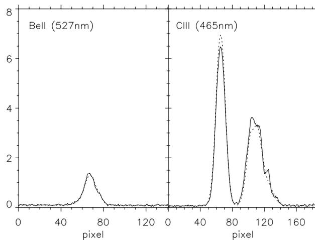
Figure 28: Measured line shape for the BeII and CIII features (solid line) and corresponding fitted modelled spectral line shape (dotted line). The fit is with contributions from the high- and low-field sides of 1:1.3 for CIII and 1:0.5 for BeII.
