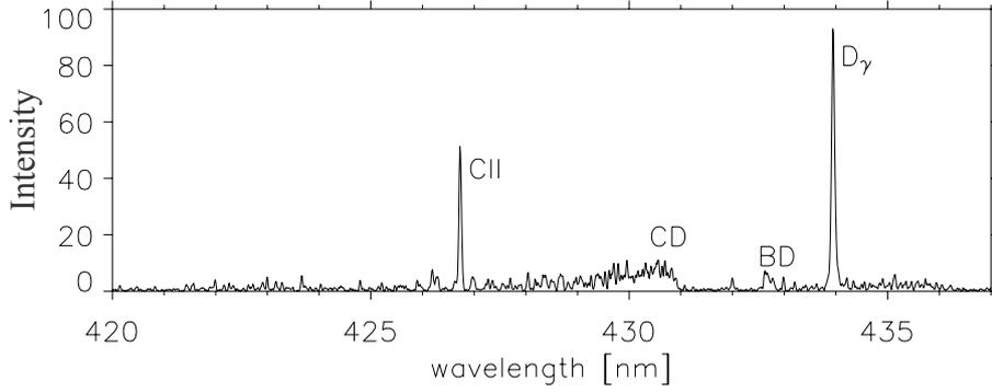
Figure 8: Section of the spectrum measured on the ASDEX Upgrade outer divertor showing the CD (Gerö) and BD molecular bands and the CII (426.7nm) and  $D_\gamma$  lines.
