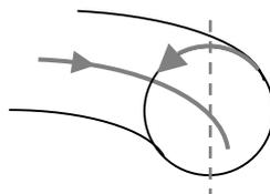
*Figure 13: The central poloidal line-of-sight (dotted line) is at right-angles to both the poloidal and toroidal components of the rotation (arrows).*
