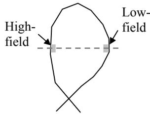
Figure 27: Sketch of the cross-section of the JET plasma showing the line-of-sight passing through the two edge emission regions, at the low and high magnetic field sides.
