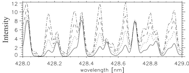
Figure 9: Variation of a section of the modelled CD spectrum with rotational temperature  $T_{rot}$  for 2500K (—); 3500K (.....); 4500K (- - -); and 5500K (-·-·-). In each case normalisation is to the 430.68nm CD band feature and one  $T_{rot}$  is assumed for all rotational levels.
