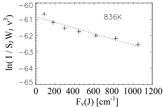
Figure 10: Boltzmann plot for  $Q$ -branch lines ( $Q2-8$ ) of the  $v=0-0$  vibrational band and linear fit revealing a  $T_{rot}$  of 836K.
