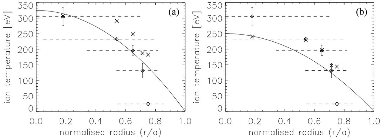
Figure 22: The modelled parabolic profile (full line) assumes (a)  $T_i(r=0)=325$ eV and (b)  $T_i(r=0)=250$ eV. The corresponding  $T_i$  calculated for each ion is given by (x) and is to be compared with the experimental  $T_i$  (◇), taking the data from the feedback case at 9.6ms. The points are plotted at the peak of the respective emissivity profiles (OII to OVI sequentially from the edge inwards) and the dashed lines represent the FWHM of the emissivity profiles.
