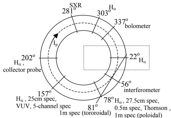
Figure 3: Schematic diagram of EXTRAP T2R top-view showing an example of the toroidal positions of spectroscopic diagnostics and the direction of the plasma current. The dotted rectangle represents the iron core. At many of the toroidal locations there are both horizontal and vertical lines-of-sight.
