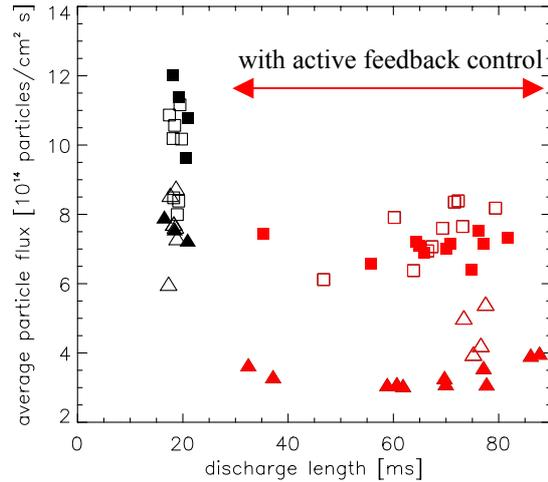
Figure 29: Particle flux results from the spectroscopic diagnostic for molybdenum ( $\Delta$ ) and chromium ( $\square$ ) in  $H_2$  (open symbols) and  $D_2$  (filled symbols) discharges. Discharges longer than 30ms have active feedback control.
