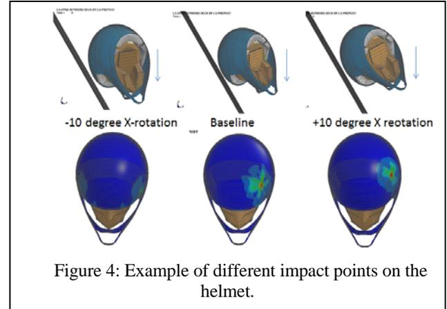
Figure 4: Example of different impact points on the helmet.
