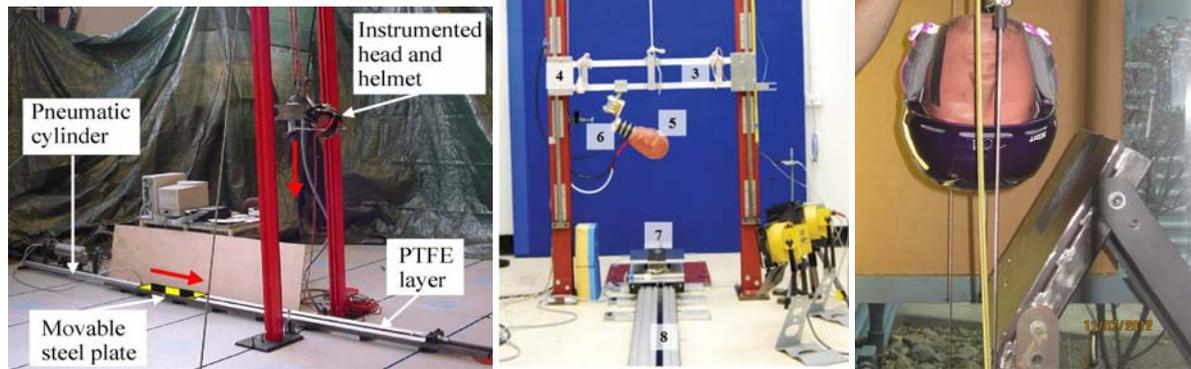
Figure 1. Different oblique test methods. Aare et al 2013, Pang et al. 2011 and photo of angled impact surface.
