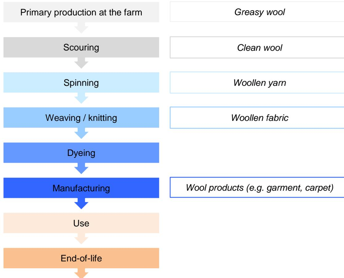
Figure 1: Simplified diagram of stages in the life cycle of wool apparel (adapted from IWTO, 2015)
