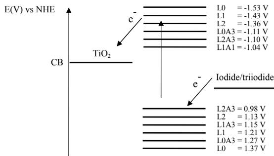
**Figure 25.** Schematic energy level diagram of the DSC and the linker series.
