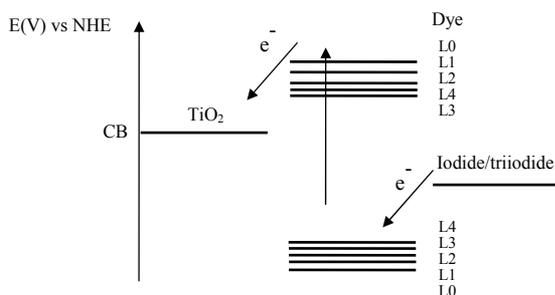
**Figure 21.** Schematic energy level diagram of the DSC and the linker series.
