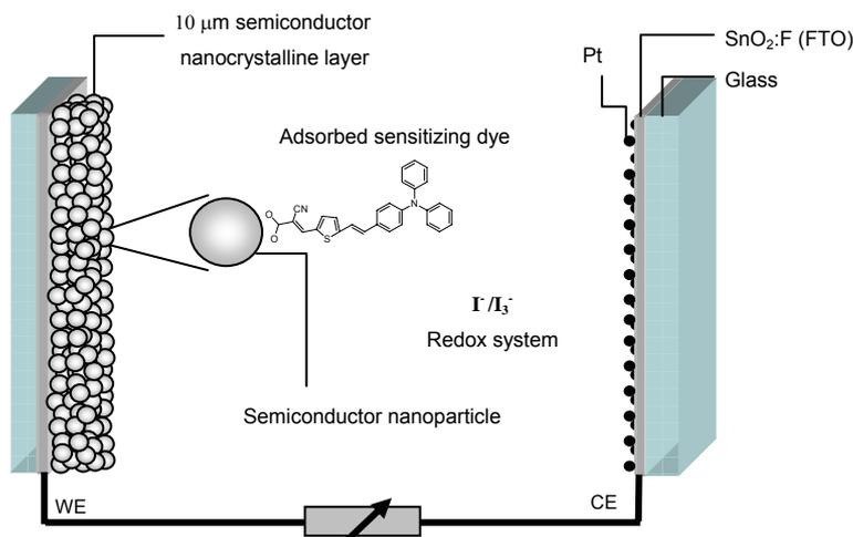
**Figure 1.** Schematic picture of the Dye Sensitized Solar Cell.
