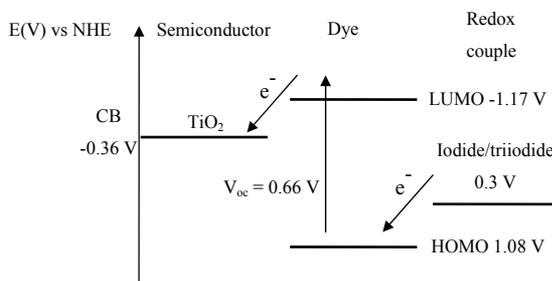
**Figure 16.** Energy level diagram of the DSC
