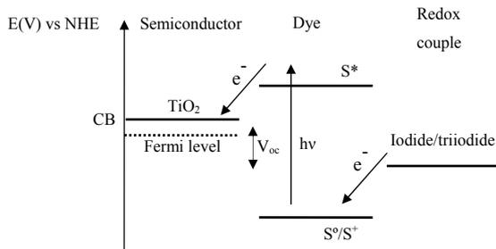
**Figure 2.** Schematic picture of the electron flow in the DSC.
