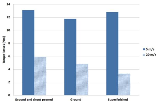
Figure 2. Influence on gear finishing and speed on torque losses.
