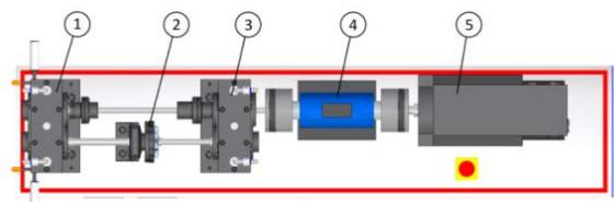
**Figure 1.** Schematic of the FZG back-to-back gear test rig with the main part marked. 1-test gearbox, 2- load clutch, 3- slave gearbox, 4- torque and speed sensor, 5- motor.
