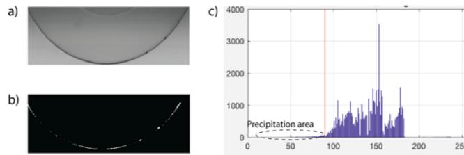
Fig.3 Image analysis code using MATLAB to convert a) original image to b) binary image, based on selection of a threshold value, c) in the histogram the entire area to the left of the threshold value was summed to evaluate the precipitation area.
