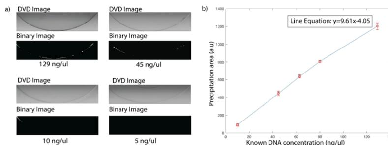
Fig.4 a) DVD generated images of a known PCR product. b) Precipitation area vs. known DNA concentration for the generated images.
