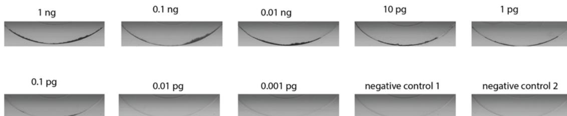
Fig.5 Images generated from DVD with eight serials 10 fold dilutions of plasmid DNA starting with a template concentration of 1 ng in 10 μl and two negative controls. Images generated for each of these sample concentrations of DNA shown. Negative control 1 denotes the LAMP assay without primers but DNA polymerase while negative control 2 depicts the absence of both primers and DNA polymerase.
