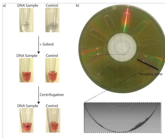
*Fig.2 a) Qualitative detection of DNA in Eppendorf tubes upon addition of GelRed followed by centrifugation. b) Generated image of the precipitate formed on the DVD.*
