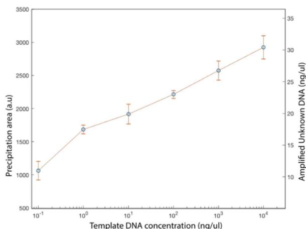
Fig.6 Starting DNA template concentration vs. precipitation area calculated from triplicate images using the MATLAB based image processing code (left-hand y-axis). Starting DNA template concentration vs. actual yield of amplified DNA produced due to the LAMP reaction (right-hand y-axis).
