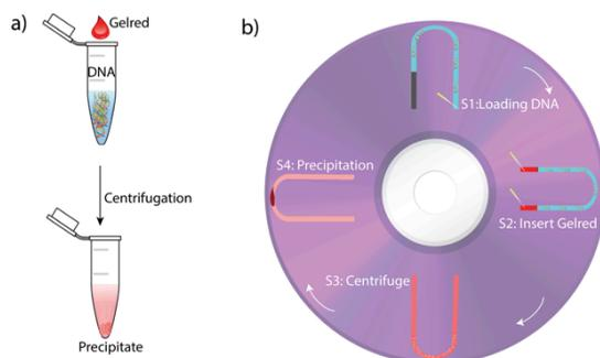
*Fig.1 Schematics of the precipitation process. a) Sample of DNA in contact with GelRed in a test tube, forms a high-density complex which precipitates upon centrifugation. b) Precipitation steps on the DVD. Step 1: loading DNA into a U-shaped channel, Step 2: inserting GelRed, Step 3: centrifuging, Step 4: formation of precipitate.*
