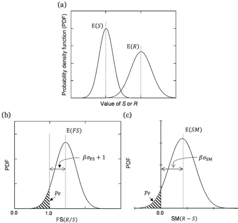
Figure 3.1. Probability distributions for (a) load ( $S$ ) and resistance ( $R$ ); (b) factor of safety ( $FS$ ); (c) safety margin ( $SM$ ).
