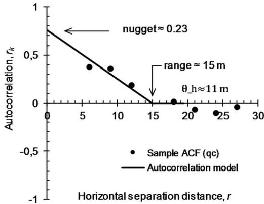
Figure 2.5. Example of an horizontal autocorrelation structure based on  $q_c$  data (Paper B, Lingwanda et al. 2017. © 2017 Taylor & Francis. Reused with permission)
