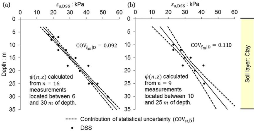
Figure 2.2. Example on the contribution from statistical uncertainty in the assessment of inherent variability of  $s_u$  from measurements of DSS; (a) 16 measurements located between 6 and 30 m of depth; (b) 9 measurement located between 10 and 25 m of depth.
