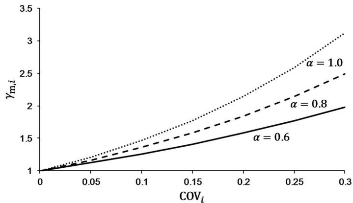
Figure 4.1. Relationship between  $\gamma_{m,i}$  and  $COV_i$  for normally distributed variables.
