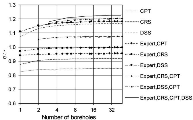
Figure 4. The  $\eta$  in relation to number of boreholes and to different combinations of site-investigation methods performed in the case project.
