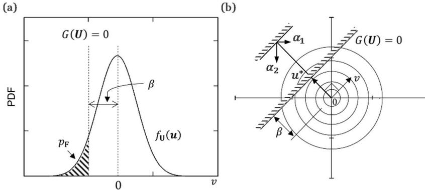
Figure 3.2. Graphical representation of the reliability index, (a) joint probability distribution  $f_U(\mathbf{u})$  of the linear limit state function in the space of the standardised normal variables; (b) contours of the joint probability distribution  $f_U(\mathbf{u})$  in the 2-dimensional standard normal space.
