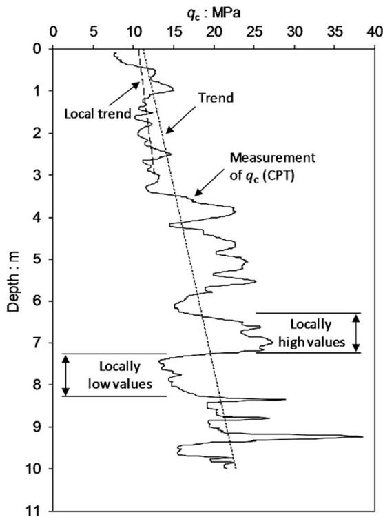
Figure 2.4. Example of fluctuations in  $q_c$  data (modified from Paper B, Lingwanda et al. 2017)
