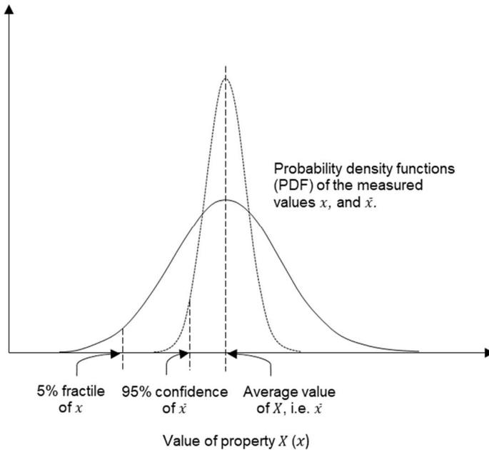
Figure 4.2. Graphical representation of the characteristic value for local and non-local failure.
