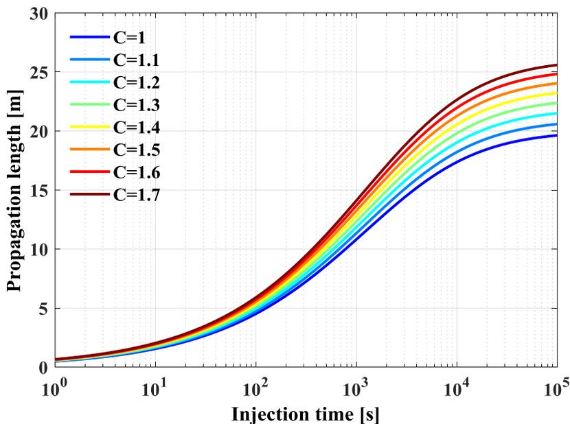
Figure 2. Illustration of the cement grout propagation with injection time for different values of the coefficient  $C$  in Hakami's model.
