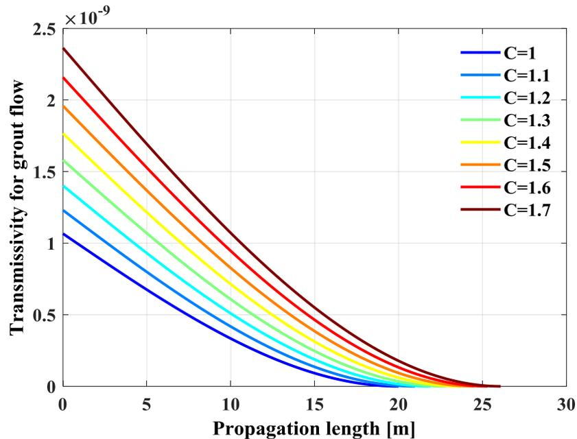
Figure 1. Illustration of the effective transmissivity for cement grouts flow in the injection process for different values of the coefficient  $C$  in Hakami's model.
