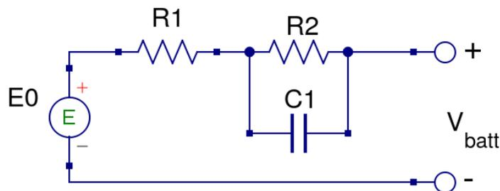
Figure 1: Randle model for a Lead-acid Battery
