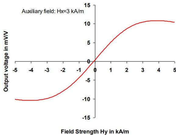
Figure 2: Output characteristics from magnetic field sensor
