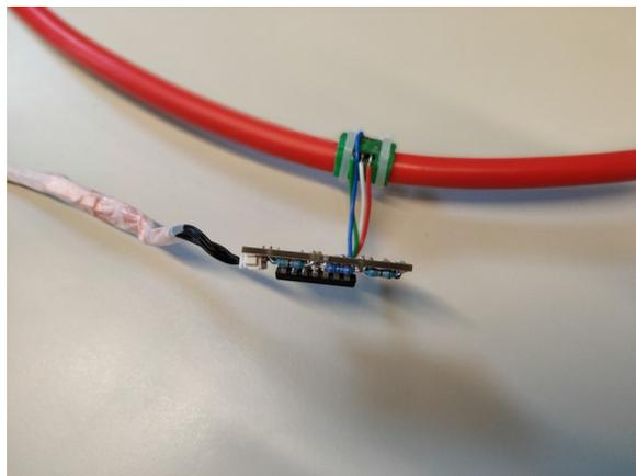
Figure 10: 3D-printed case for sensor with amplifier circuit.
