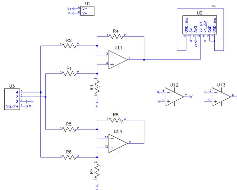
Figure 4: The differential amplifier for the magnetoresistive sensor.
