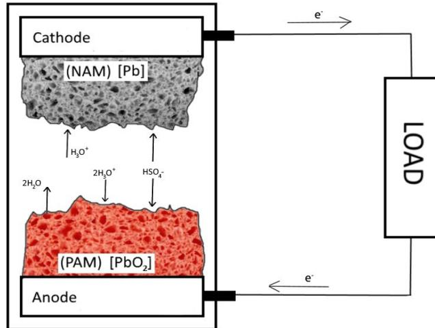
Figure 8: Illustration of the chemical reactions inside a lead-acid battery.
