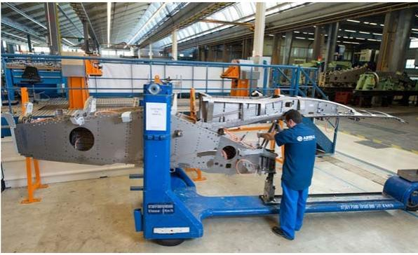
Figure 2. Photo of an assembled engine pylon [3]
