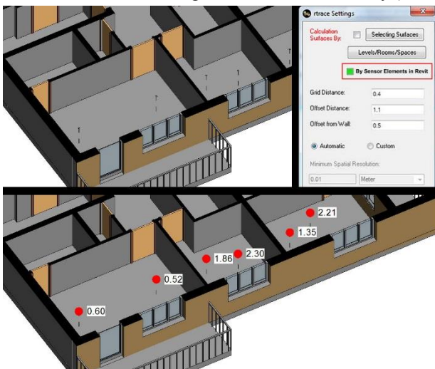
Figure 5: Creating calculation points with the help of placing one type of Generic-Model Revit Family and presenting its results in Revit with this add-in
