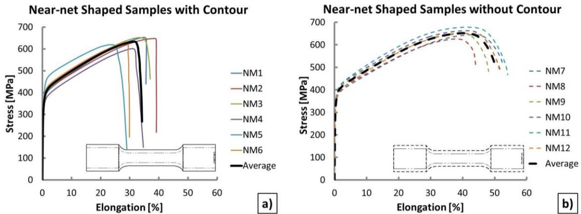
Fig. 4 Tensile properties of samples printed (a) with contour and (b) without contour and machined from near-net shaped samples.
