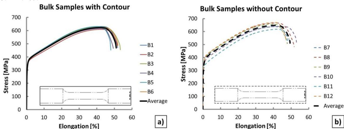
Fig. 3 Tensile properties of samples EBMed (a) with contour and (b) without contour and deeply machined from bulk cylinders.
