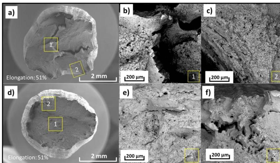
Fig. 5 Typical fracture surfaces of bulk samples; With Contour: a), fracture surface; b), location 1; c), location 2. Without Contour: d), fracture surface; e), location 1; f), location 2
