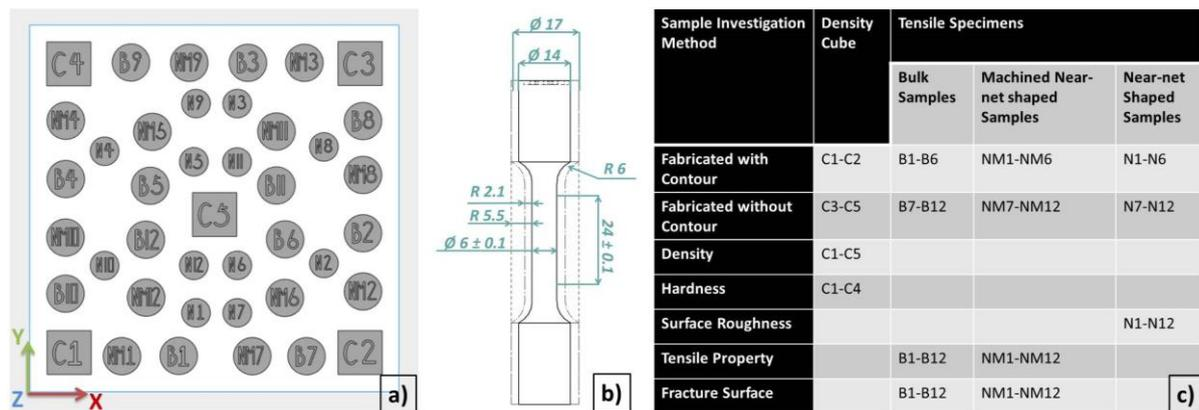
Fig. 1: (a) Layout of the built, (b) dimension of the tensile specimens; dash, center, and solid lines represent the bulk, the near-net shaped, and the samples after machining respectively, and (c) summary of the coded samples.
