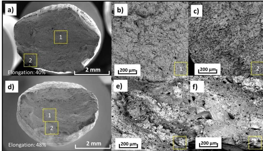
Fig. 6 Typical fracture surfaces of near-net shaped samples; With Contour: a), fracture surface; b), location 1; c), location 2. Without Contour: d), fracture surface; e), location 1; f), location 2
