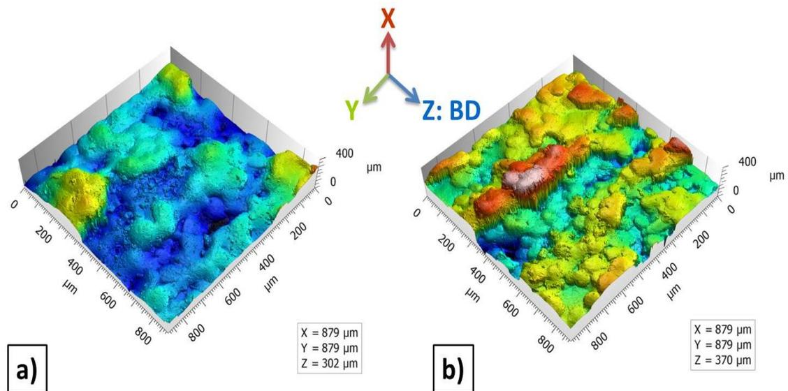
Fig. 2 The surfaces of a) sample C1 with contour and b) sample C4 without any contour.
