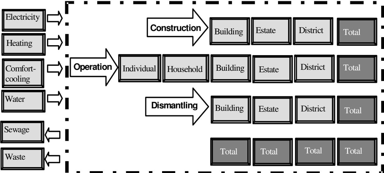
**Figure 2.** The different levels in the ELP (i.e. building level, estate level and district level), the life cycle perspective (i.e. construction, operation and development) and the inputs and outputs to a building, an estate or a district (e.g. electricity and heat).
