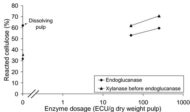
**Fig 8.** Reactivity, according to Fock, of sequential enzymatic treatment for eucalypt kraft pulp at different endoglucanase dosage (represented in a logarithmic scale). Endoglucanase dosage: 0, 50 and 250 ECU/g dry weight pulp at 1 h incubation time. Xylanase dosage: 500 EXU/g dry weight pulp at 2 h incubation time.
