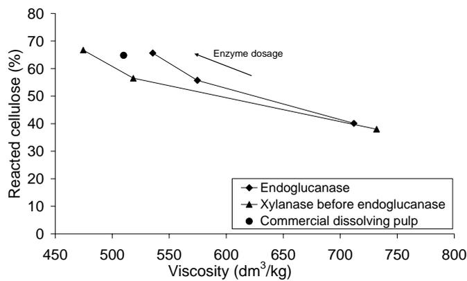
**Fig 9.** Relation between reacted cellulose and viscosity for birch pulp. Endoglucanase dosage: 0, 50 and 250 ECU/ g dry weight pulp. Xylanase dosage: 500 EXU/ g dry weight pulp.
