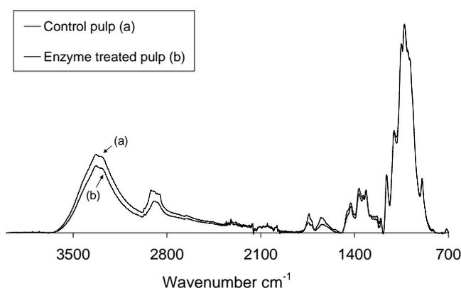
**Fig 3.** FTIR spectra for birch pulp treated with 250 ECU/g dry weight pulp endoglucanase and the control pulp. Incubation time: 1 h.
