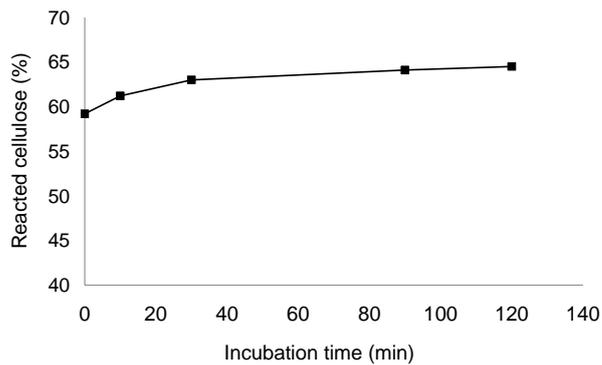
**Fig 3.** Reactivity of enzyme-treated dissolving pulp, according to Fock, as a function of incubation time. Enzyme dosage: 30 ECU/g dry weight pulp.
