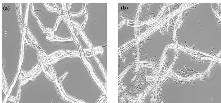
**Fig 4.** Commercial dissolving pulp: (a) untreated, and (b) after being subjected to an intensive mechanical treatment.
