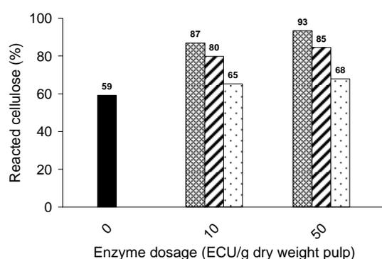
**Fig 8.** The cellulose reactivity, according to Fock for N476 (■), N51063 (▨) and N613 (□) at two enzyme dosages and a control pulp without enzymatic treatment (■). Incubation time: 1 h.
