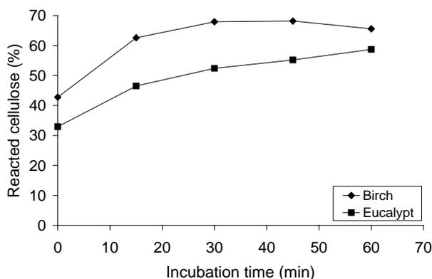
**Fig 5.** Reactivity of enzyme-treated birch and eucalypt kraft pulps, according to Fock, as a function of incubation time. Enzyme dosage: 250 ECU/g dry weight pulp.
