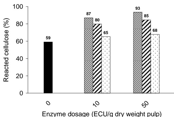
**Fig 7.** Comparison of the cellulose reactivity, according to Fock, among N476 (▨), N51063 (▩), N613 (□) and a control pulp (■). Incubation time: 1 h.
