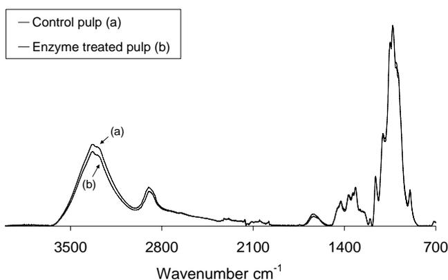
**Fig 4.** FTIR spectra for eucalypt pulp treated with 250 ECU/ g dry weight pulp endoglucanase and the control pulp. Incubation time: 1 h.
