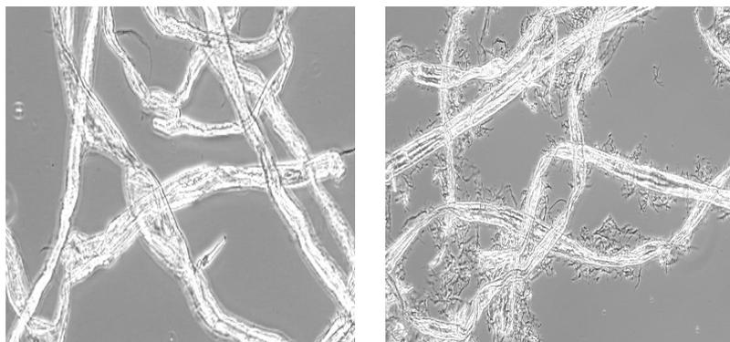
**Fig 4.** Commercial dissolving pulp: untreated (left) and, after being subjected to an intensive mechanical treatment (right).
