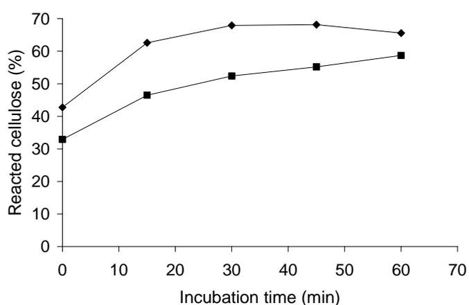
**Fig 9.** Reactivity, according to Fock, of the birch-treated pulp (◆) and eucalypt-treated pulp (■) as a function of the incubation time. Enzyme dosage: 250 ECU/g dry weight pulp.
