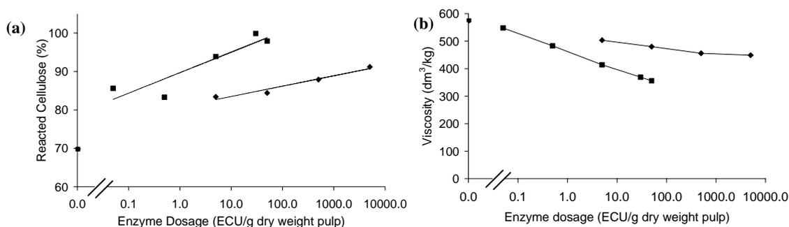
**Fig 3.** (a) Reactivity, according to Fock, after enzymatic treatment. (b) Pulp viscosity after enzymatic treatment. The enzymatic treatments were done with: (■) a monocomponent endoglucanase with a CBD (N476) and (◆) a monocomponent endoglucanase without a CBD (N613). Incubation time: 1 h. Enzyme dosages for N613: 0, 5, 50, 500, and 5000 ECU/g dry weight pulp. Enzyme dosages for N476: 0, 0.05, 0.5, 30, and 50 ECU/g dry weight pulp. The values for N476 were taken from a previous study [22].
