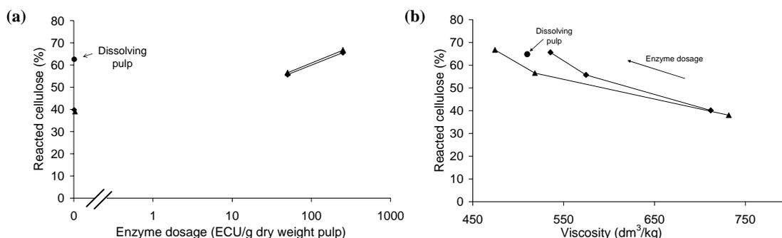
**Fig 12.** (a) Cellulose reactivity of birch pulp as a function of the enzyme dosage and (b) viscosity of the pulp after a treatment with: (◆) endoglucanase and (▲) xylanase prior to endoglucanase. Incubation time for endoglucanase: 1 h, and for xylanase: 2 h. Enzyme dosage: 0, 50, and 250 ECU/g dry weight pulp.
