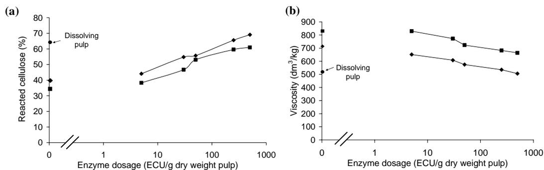
**Fig 8.** (a) Reactivity, according to Fock, of the treated pulps. (b) Viscosity of the treated pulp. The (◆) represents the birch pulp and the (■) represents the eucalypt pulp. Enzyme dosage: 0, 5, 50, 500, and 5000 ECU/g dry weight pulp. Incubation time: 1 h.
