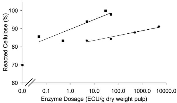
**Fig 1.** Reactivity according to Fock method after enzymatic treatment with a monocomponent endoglucanase with CBD (N476) (■) and CBD-free (N613) (◆). Incubation time: 1 h. The values for N476 are taken from a previous study [4].
