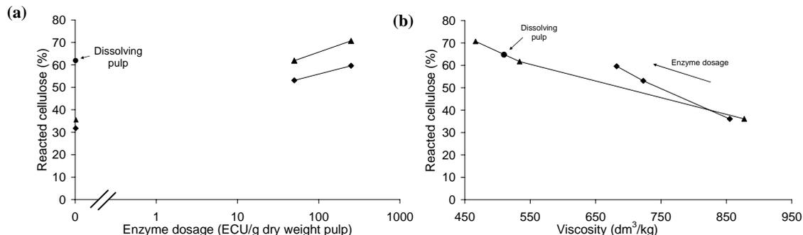
**Fig 13.** (a) Cellulose reactivity of eucalypt pulp as a function of the enzyme dosage and (b) viscosity of the pulp after a treatment with: (◆) endoglucanase and (▲) xylanase prior to endoglucanase. Incubation time for endoglucanase: 1 h, and for xylanase: 2 h. Enzyme dosage: 0, 50, and 250 ECU/g dry weight pulp.
