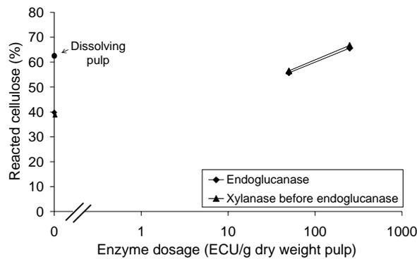
**Fig 7.** Reactivity, according to Fock, of sequential enzymatic treatment for birch kraft pulp at different endoglucanase dosages (represented in a logarithmic scale). Endoglucanase dosage: 0, 50 and 250 ECU/g dry weight pulp at 1h incubation time. Xylanase dosage: 500 EXU/g dry weight pulp at 2 h incubation time.
