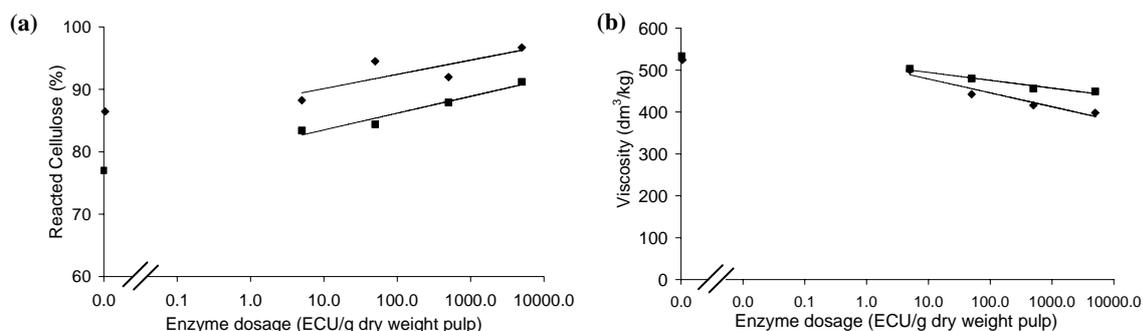
**Fig 5.** (a) Reactivity, according to Fock, of the treated pulp. (b) Viscosity of the treated pulp. The pulp was subjected to (■) enzymatic treatment with N613 only and (◆) intensive mechanical treatment followed by enzymatic treatment with N613. Enzyme dosage: 0, 5, 50, 500, and 5000 ECU/g dry pulp. Incubation time: 1 h.
