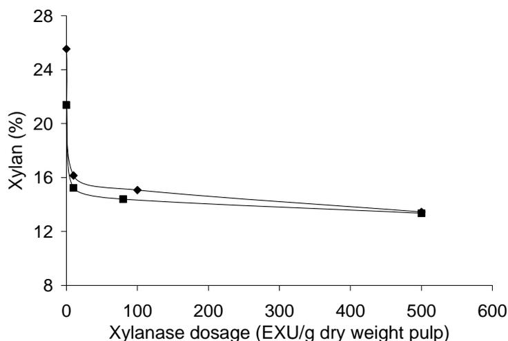
**Fig 11.** Reduction of xylan content of birch (◆) and eucalypt (■) kraft pulps as a function of the enzyme dosage. Incubation time: 2 h.
