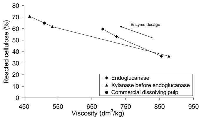
**Fig 10.** Relation between reacted cellulose and viscosity for eucalypt pulp. Endoglucanase dosage: 0, 50 and 250 ECU/ g dry weight pulp. Xylanase dosage: 500 EXU/ g dry weight pulp.
