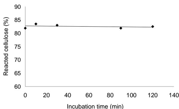
**Fig 7.** Reactivity of mechanically and enzymatically treated dissolving pulp, according to Fock, as a function of the incubation time. Enzyme dosage: 30 ECU/g dry weight pulp.
