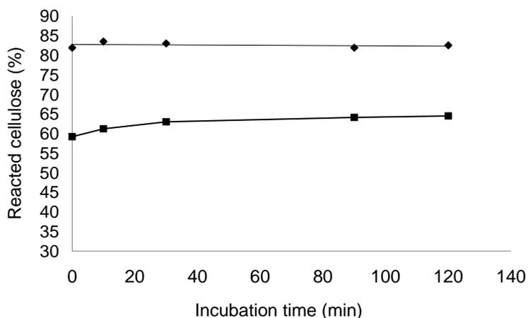
**Fig 6.** Reaction time of N613 towards the dissolving pulp with: (■) only enzymatic treatment and (◆) an intensive mechanical treatment followed by enzymatic treatment. Enzyme dosage: 30 ECU/g dry weight pulp.
