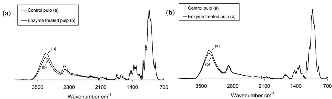
**Fig 10.** (a) FTIR spectrum for birch pulp. (b) FTIR spectrum for eucalypt pulp. Enzyme dosage: 250 ECU/g dry weight pulp. Incubation time: 1 h.
