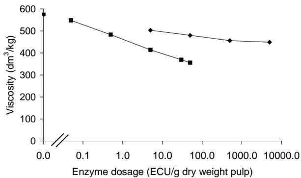
**Fig 2.** Pulp viscosity after enzymatic treatment with N476 (■) and N613 (◆). Incubation time: 1 h. The values for the N476 were taken from a previous study [4].
