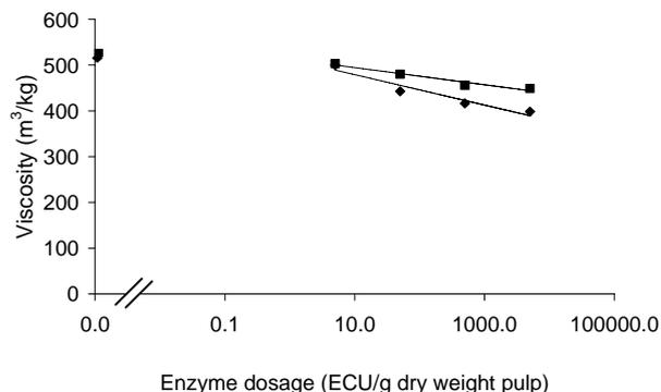
**Fig 6.** Comparison in viscosity of a commercial dissolving pulp subjected to (■) enzymatic treatment with a N613 only and (◆) intensive mechanical treatment followed by enzymatic treatment with a N613. Enzyme dosage: 5, 50, 500, 5000 ECU/g dry pulp. Incubation time: 1 h.
