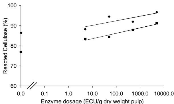
**Fig 5.** Reactivity according to the Fock method of a commercial dissolving pulp subjected to (■) enzymatic treatment with N613 and (◆) intensive mechanical treatment followed by enzymatic treatment with N613. Enzyme dosages: 5, 50, 500, 5000 ECU/g dry pulp. Incubation time: 1 h.
