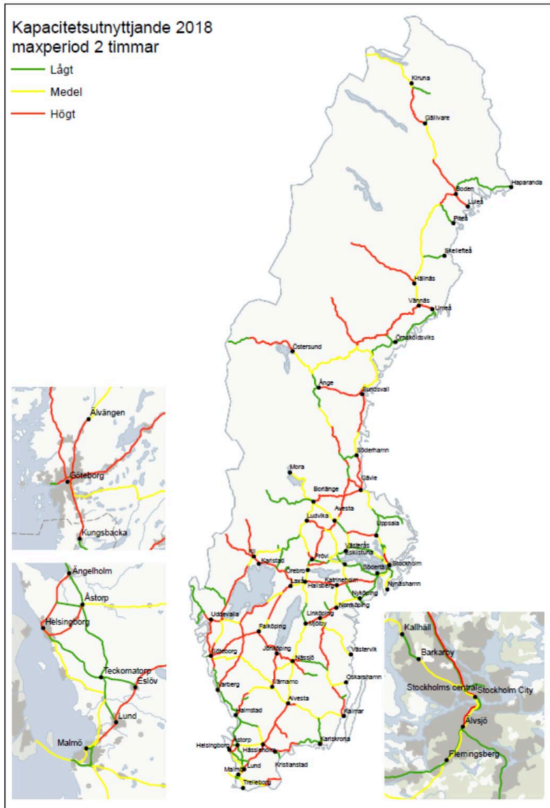
Figure 1: Rail capacity usage in Sweden in 2018 during peak times. Extracted from Trafikverket (2018a) 1
