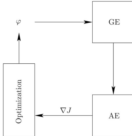
FIGURE 3.1. The optimization procedure. The control is denoted  $\varphi$ . The gradient of the objective function with respect to the control  $\varphi$  is denoted  $\nabla J$  where  $J$  is the objective function. The governing equations and associated adjoint equations are denoted GE and AE respectively.
