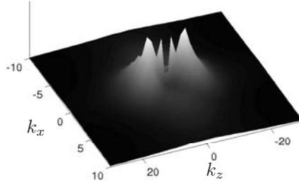
FIGURE 2.4. Maximum amplitude of turbulent covariance data as a function of wavenumber pair  $\{k_x, k_z\}$ . The corresponding two-point correlations along the wall-normal coordinate are shown in figure 2.2.
