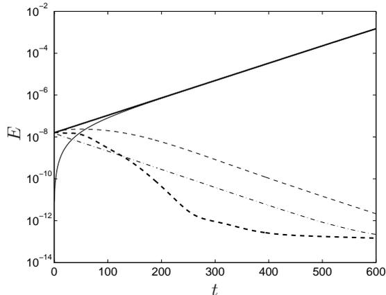
FIGURE 2.8. Time evolution of the perturbation energy of the uncontrolled unstable eigenmode at  $\alpha = 0.25, \beta = -0.25$  in a Falkner–Skani–Cooke boundary layer and the corresponding controlled system. Solid: uncontrolled energy growth. Dashed: full information control is applied. Solid-thin: energy growth in the estimator when no control is applied. Dash-dotted-thin: the estimation error when no control is applied. Dashed-thin: compensator control is applied.
