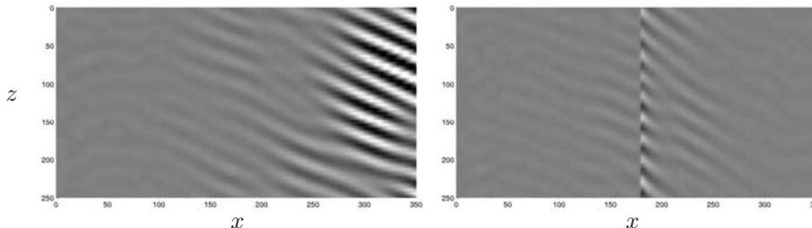
FIGURE 2.10. Snapshots of the wall-normal velocity component at  $y = 0.5$ . The flow state is depicted in part (a). In (b) the effect of the compensator control is shown. In the controlled flow the control has been applied for 2000 time units i.e. all the transient effects that occur due to the startup of the control with the perturbations present have settled down. The control is applied in  $x \in [175, 325]$ . The black to white scale lies in the interval  $v \in (-0.00045, 0.00045)$ .
