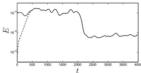
FIGURE 2.11. *Time evolution* of the disturbance energy integrated throughout the computational box. During the first 2000 time units the flow is uncontrolled. At time  $t = 2000$  the compensator control is turned on. Solid: energy in the “real” flow. Dashed: energy in the estimator.
