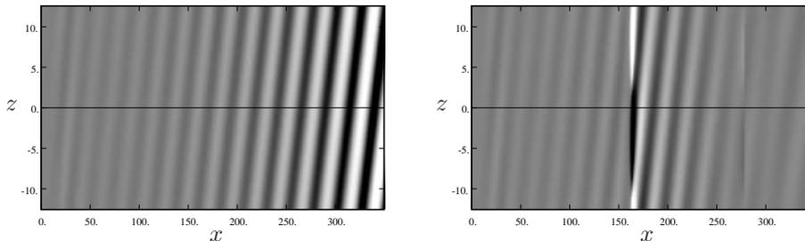
FIGURE 3.2. Snapshot of the wall normal velocity component in an  $x$ - $z$  plane at  $y = 0.5$  without control (left) and with nonlinear control (right). The control is applied in  $x \in (145, 295)$ . The black to white scale lies in the interval  $v \in (-0.001, 0.001)$ .
