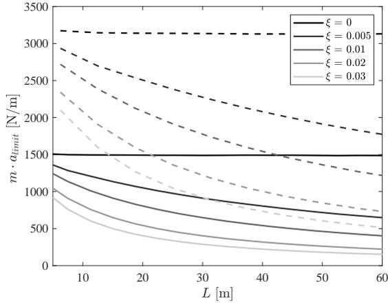
Figure 4.6: Minimum linear mass as a function of span length (—normal running —normal walking).
