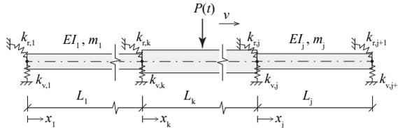
Figure 4.7: A continuous beam system on elastic supports as in Paper I.
