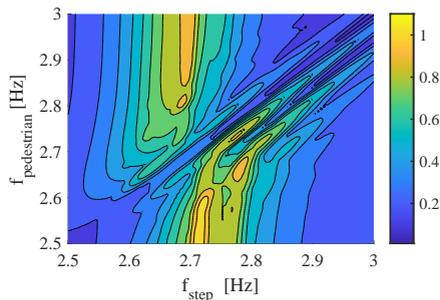
Figure 4.3: Acceleration response surface, KTH Bridge. [ $\text{m/s}^2$ ].
