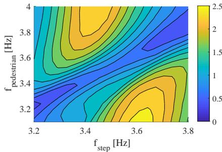
Figure 4.2: Acceleration response surface, Vega Bridge. [ $\text{m/s}^2$ ].
