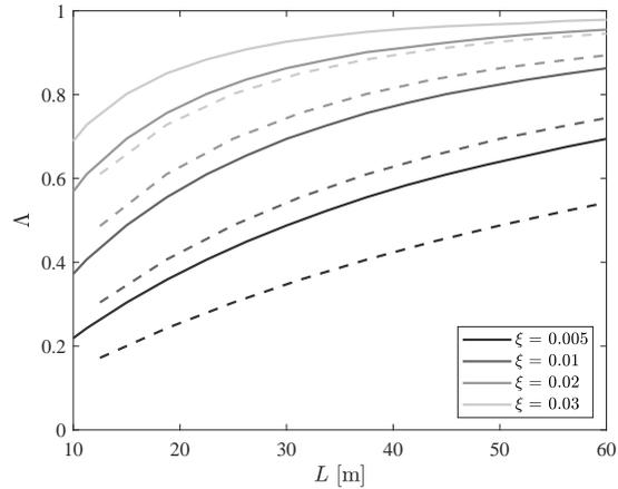
Figure 4.5: The parameter  $\Lambda$  as a function of span length (- -normal running —normal walking).
