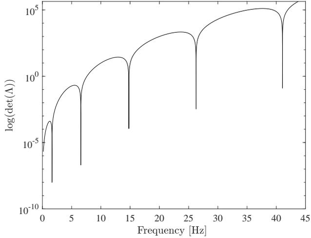
Figure 4.8: Frequencies of Example 1: Simply supported bridge.
