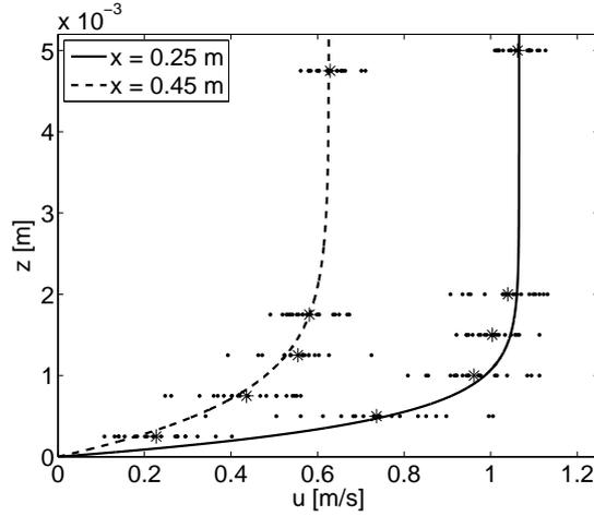
FIGURE 4. Theoretical velocity profiles for  $x = 0.24$  m (solid) and  $x = 0.45$  m (dashed). The dots and the stars denotes the velocities of individual fibres and the mean of all fibres in each particular serie, respectively.
