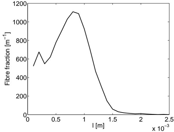
FIGURE 3. Length distribution of fibres in the suspension.
