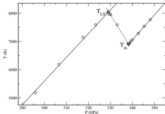
FIG. 1: Example of the application of the Z-method to determine the melting temperature. The relation between  $T_m$  (lower point of the Z-shaped isochoric curve) and  $T_{LS}$  (higher point) is shown for an embedded-atom solid.
