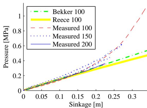
Figure 5.16: Measured pressure and sinkage on loose sand. All measured data are shown in the figure, but the estimated models are based on sinkages down to 0.14 m. Predictions are only shown for the smallest sinkage plate since the predictions for larger sinkage plates coincide and cannot be discerned from the smallest sinkage plate.
