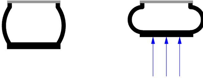
Figure 3.11: Tyre cross section with flexible sidewalls and rigid tread. Equilibrium without ground pressure to the left, deformation as ground pressure is applied to the right.
