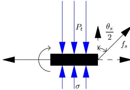
Figure 3.12: Free body diagram for the rightmost half part of the tread of a tyre.
