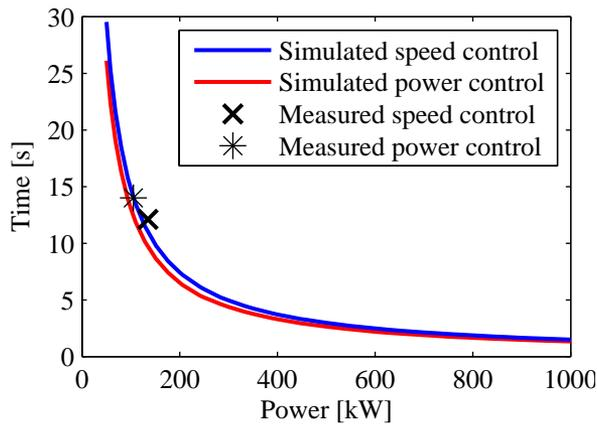
Figure 5.5: Pivot turning time is depending on available power.
