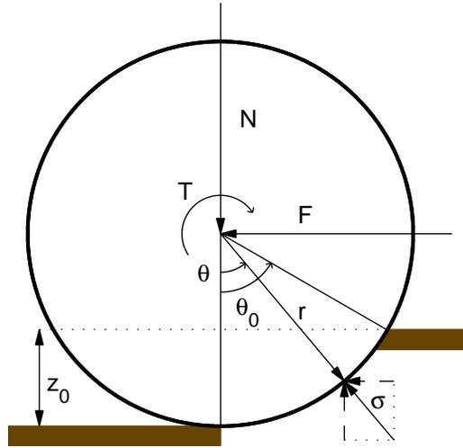
Figure 3.7: Model for driven wheel on soft ground.
