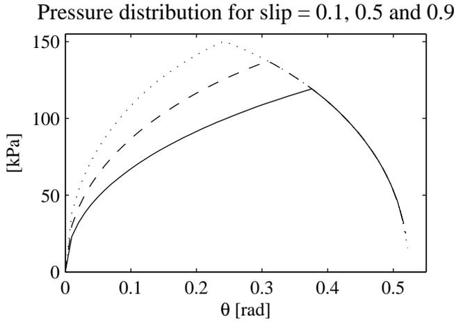
Figure 3.8: The pressure distribution beneath the tyre contact area for slip 0.1 (dotted line), 0.5 (dashed line) and 0.9 (solid line). In this case  $\theta_0$  is set to be the same independently of the slip and the vertical force due to the ground pressure will thereby be reduced as the slip is increased.
