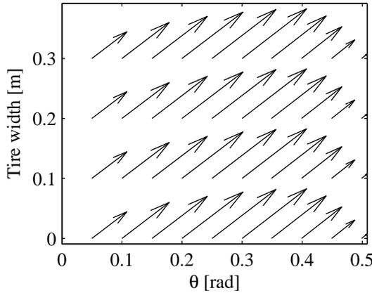
Figure 3.9: Shear stresses beneath the tyre contact area for  $s = 0.5$ ,  $\alpha = 0.2$  rad. The y-axis represents the width of the tyre and the x-axis represents the longitudinal direction of the contact area. Zero corresponds to the point below the wheel centre and in this case  $\theta_0 = 0.5$  rad.
