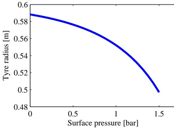
Figure 3.14: Tyre radius versus surface pressure for tyre pressure of 1.5 bar. Although the surface pressure on the tyre does not exceed the tyre pressure, there is a significant deformation of the tyre.
