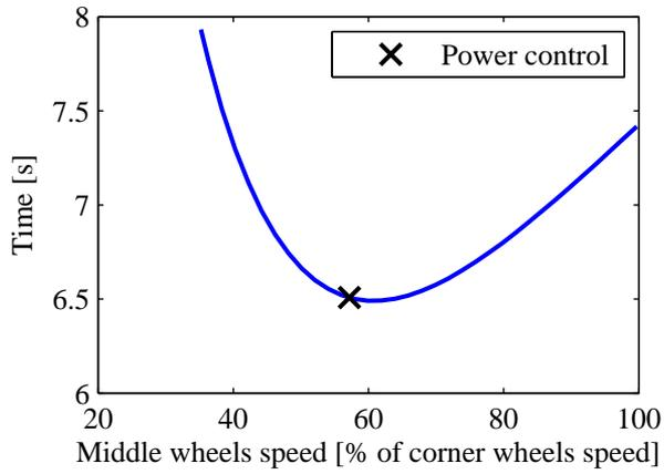
Figure 5.6: Keeping the total power consumption constant, the middle wheels should be run slower than the corner wheels to minimise the pivot turning time.
