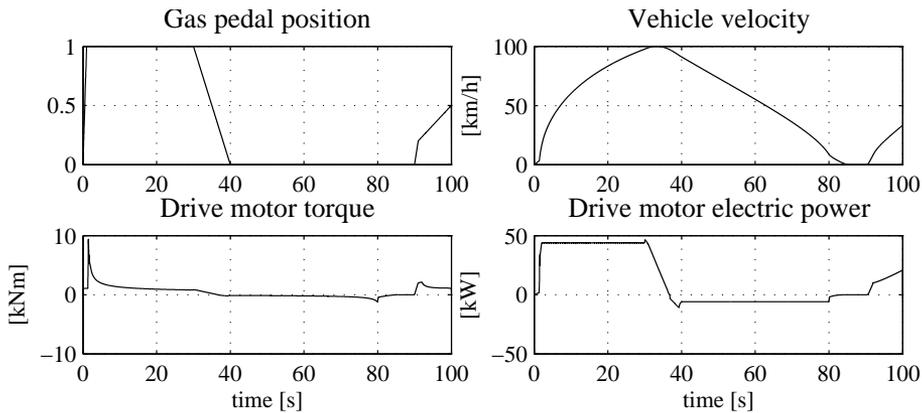
Figure 5.11: Gas pedal position (1 corresponds to full gas, 0 is released gas pedal), vehicle velocity, drive motor torque and drive motor electric power.
