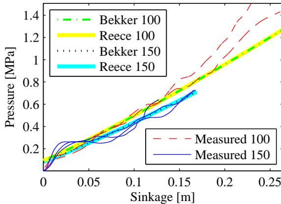
Figure 5.15: Measured pressure and sinkage on compact sand. All measured data are shown in the figure, but the estimated models are based on sinkages down to 0.14 m.
