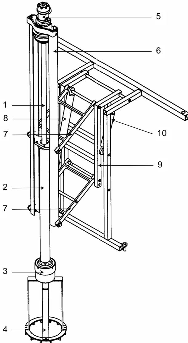
Figure 4.1: Drawing of Bevameter used for measurements.
