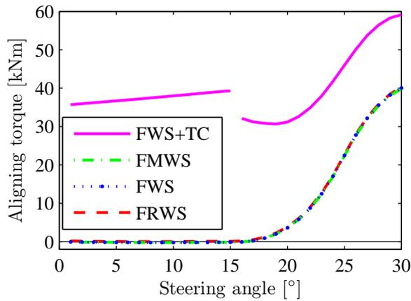
Figure 5.10: Aligning yaw torque for different steering methods,  $\beta = 25^\circ$  and  $\mu_s = 0.3$ .
