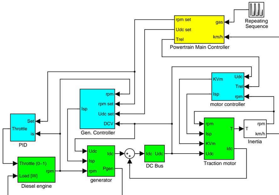
Figure 3.5: Model for the complete electric transmission system.
