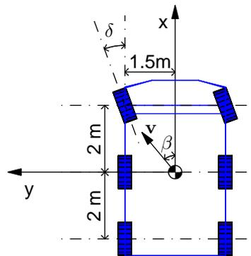
Figure 3.4: Vehicle geometry and definition of  $\beta$ .
