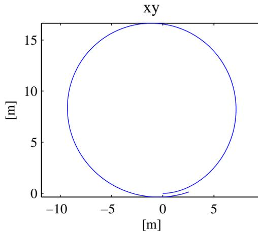
Figure 5.14: Vehicle path when turning on soft ground using both front and rear wheel steering. The torque of the wheels are determined by a speed controller.
