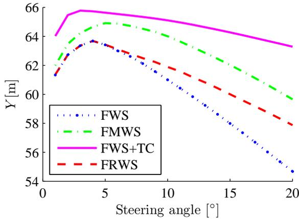
Figure 5.9:  $Y$  position at  $X = 300$  m vs. steering angle during a J-turn for different vehicle steering configurations and  $\mu_s = 0.1$ .
