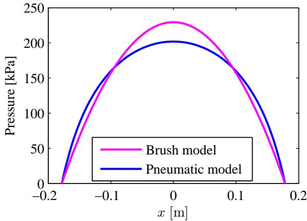
Figure 5.2: Different models for longitudinal pressure distribution in the contact area.
