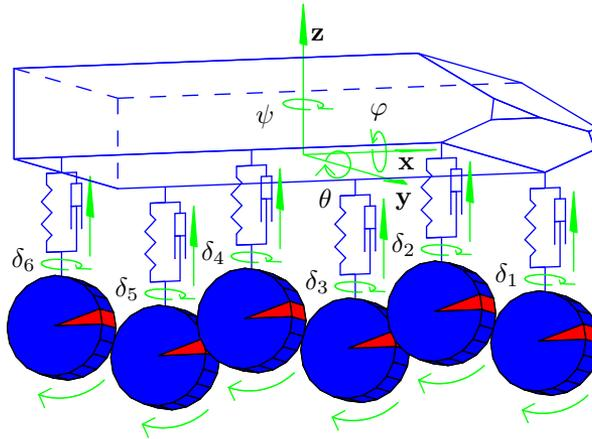
Figure 3.3: Complete vehicle model with springs and dampers. The vehicle model has 24 DOF, excluding the tyre model.
