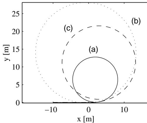
Figure 5.3: J-turn turning paths with the three different steering methods (a) front and rear, (b) front and middle and (c) only front wheels.
