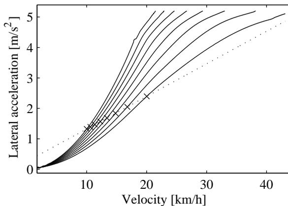
Figure 5.4: Lateral acceleration for  $20^\circ$  steering angle on the front wheels and different steering angles on the rear wheels.
