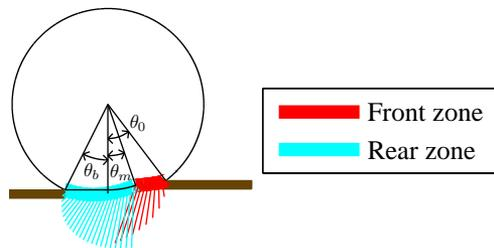
Figure 3.15: Side profile of flexible tyre on soft ground. The lines beneath the wheel show the resultant of the ground pressure and shear stresses in the rear and front zone.
