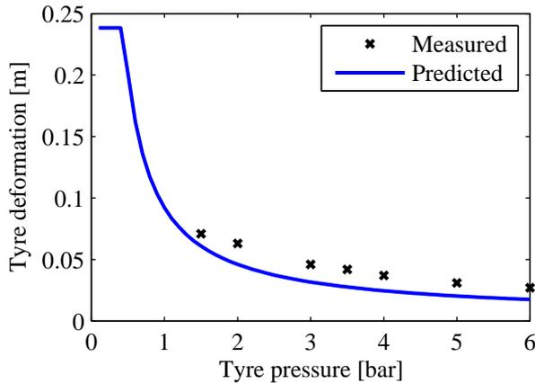
Figure 5.1: Deformation for a tyre on flat, rigid ground.
