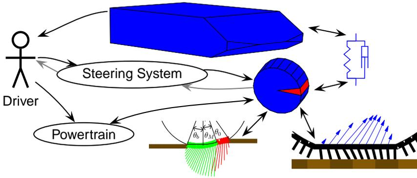
Figure 3.1: Schematic figure of the complete model. Depending on the vehicle, some of the subsystems should be multiplied. The vehicle considered in this work contains six wheels with drive motors and two diesel engines with generators.
