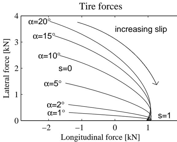
Figure 3.10: Longitudinal and lateral forces when the slip is varied from 0 at the left part of the lines to 1 at the lower right end of the lines at different steering angles.
