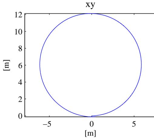
Figure 5.13: Vehicle path when turning on soft ground using both front and rear wheel steering and equal torque on all wheels.
