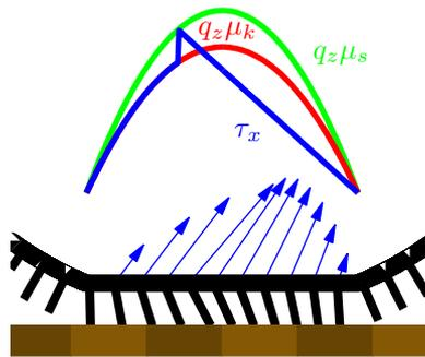
Figure 3.6: Shear stress and normal load distribution in the brush tyre model for pure longitudinal slip.
