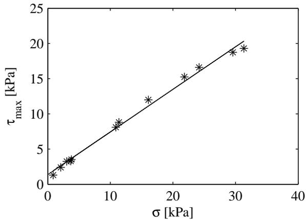
Figure 5.17: Measured maximum shear stress at different ground pressures (\*) and a least squares fit (-).
