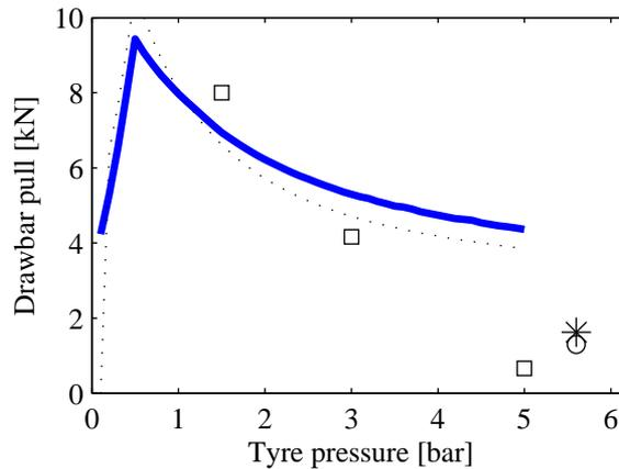
Figure 5.19: Simulated drawbar pull on prepared sand bed (—) at varying tyre pressure. Simulated drawbar pull on loose sand (···), measured drawbar pull (□) and simulated drawbar pull for a rigid wheel on prepared sand (⊙) and loose sand (\*) are also shown.
