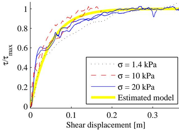
Figure 5.18: Measured maximum shear stress at different ground pressures and a least squares fit model.
