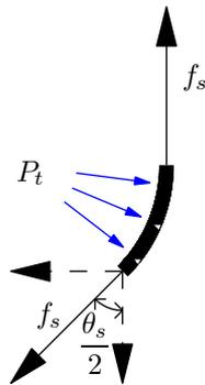
Figure 3.13: Free body diagram for the lower part of the tyre sidewall.
