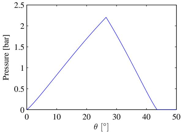
Figure 5.20: Normal stresses beneath a rigid wheel with 2250 kg vertical load at 30 % slip.
