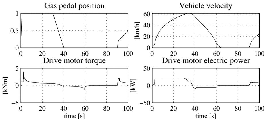
Figure 5.12: Gas pedal position (1 corresponds to full gas, 0 is released gas pedal), vehicle velocity, drive motor torque and drive motor electric power with reduced performance on diesel engine.
