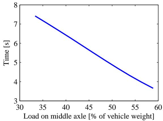
Figure 5.7: The pivot turning time is reduced when more load is distributed to the middle wheels.
