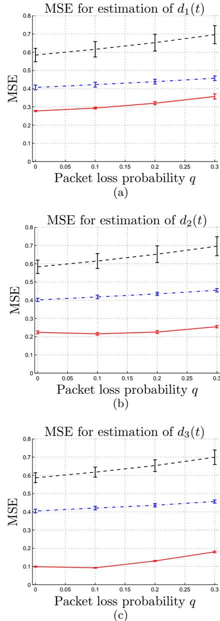
Figure 4: Mean Square Error (MSE) performance comparison among estimators for various i.i.d. packet loss probabilities  $q$  for a network with  $N = 10$  nodes. Each plot is associated to one of the three test signals  $d_1(t), \dots, d_3(t)$ , see Fig. 3. The dashed line refers to the estimator  $E_1$ , the dashed-dotted line refers to the estimator  $E_2$  and the solid line to the proposed estimator  $E_p$ . The vertical bars represent the variance of the MSE computed for the 20 simulations.
