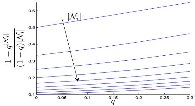
Figure 1: Eq. (5.9) (which is the second factor of (5.8) for packet losses i.i.d.) as function of  $q$  for increasing values of  $|\mathcal{N}_i|$  ranging from 2 to 10. The factor is always less than 1. The smallest values are achieved when  $q$  is small and  $|\mathcal{N}_i|$  is large. This is explained by that the packet loss probability has a decreasing negative effect when the number of neighbors of a node increases, which translates into a smaller value of the coefficient.
