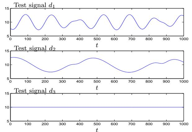
Figure 3: Test signals used to compare performance with various estimator. The signals are generated accordingly to  $d_i(t) = 3(\sin(2\pi\omega_i t/300)) + 10 - 0.5 \sin(2\pi\omega_i t/300)(1 - \exp(-t/300))/(\sin(2\omega_i \pi t/500) + 1.2)$  with  $\omega_1 = 1$ ,  $\omega_2 = 0.5$  and  $\omega_3 = 0$ .
