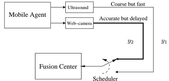
Fig. 1. The system architecture for the localization of a mobile agent using a heterogeneous sensor network.
