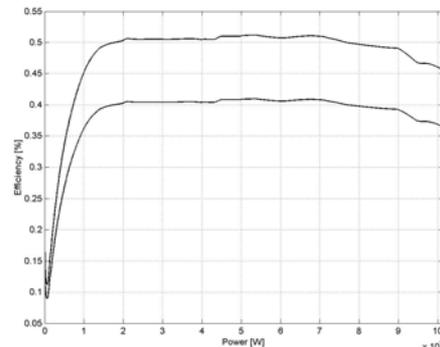
Figure 4.2. Original and up-scaled efficiency curves of the conventional combustion engine. The upscaling is done to simulate a free-piston engine.
