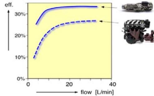
Figure 4.1. Overall efficiency of a free-piston engine pump compared to the efficiency of a comparably sized conventional diesel engine piston in-line pump [2].
