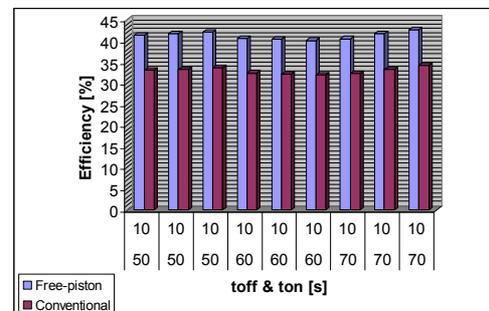
Figure 6.4. System efficiency versus time intervals  $t_{on}$  and  $t_{off}$  ( $P_{limit}=20, 28, 35$  kW, strategy 3).
