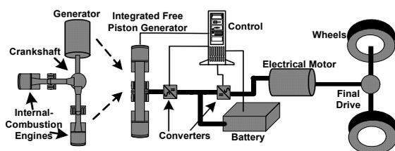
Figure 1.1. A free-piston generator fed series hybrid vehicle.
