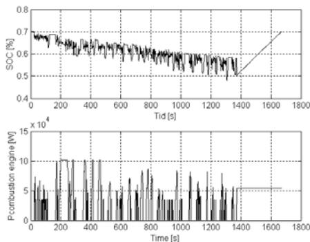
Figure 6.1. Battery state of charge and the power from the combustion engine versus time for strategy 3, without time control.
