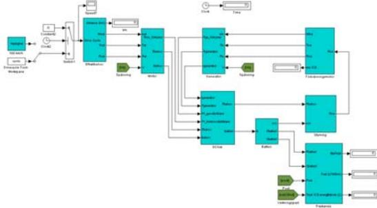
Figure 2.1. SEHV system built in a MATLAB Simulink environment.
