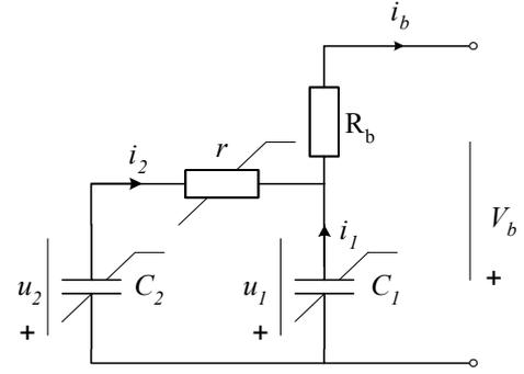
Figure 2.3. Equivalent electrical circuit of a lithium-ion cell.
