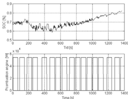
Figure 6.2. Battery state of charge and the power from the combustion engine versus time for strategy 2.
