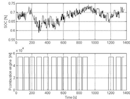
Figure 6.3. Battery state of charge and the power from the combustion engine versus time with introduced new SOC limits for strategy 2.
