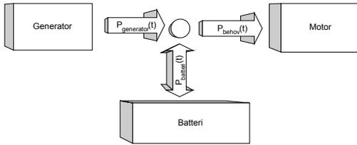
Figure 2.2. Power balance in the SEHV system.
