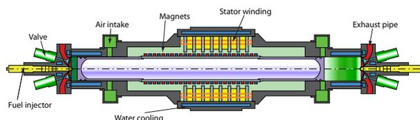
Fig. 1. Schematic view of the FPEC.
