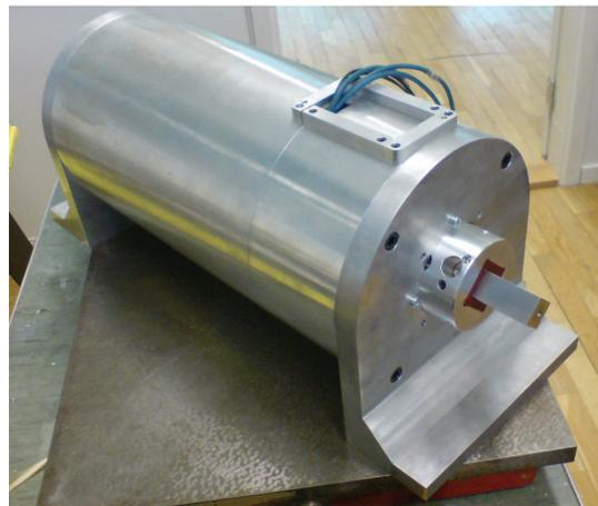
Fig. 12. Prototype of the novel linear TFM.
