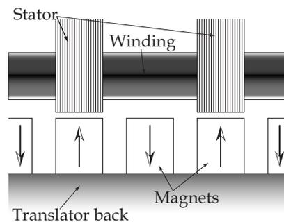
Fig. 2. Layout of the new TFM design
