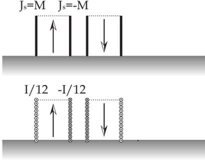
Fig. 7. Equivalent PM punctual currents.
