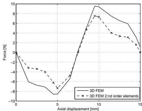
Fig. 10. 3D-simulated force for one phase magnets.
