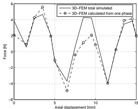
Fig. 11. 3D-simulated force for all phases and calculated results from 3D-FEM results for one phase.
