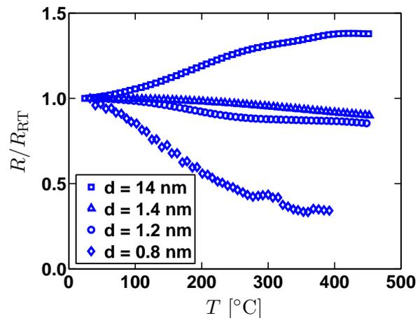
**Figure 4.** The normalized film electrical resistance  $R/R_{RT}$  versus temperature for a film grown at room temperature. The symbols correspond to the symbols marking thickness and resistance shown in figure 3.
