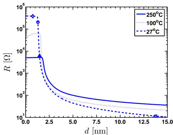
**Figure 3.** The electrical resistance,  $R$ , as a function of Pt film thickness,  $d$ , measured *in-situ* during growth, for three different growth temperatures.
