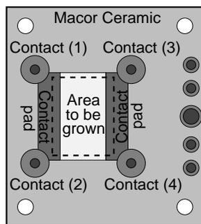
**Figure 1.** A schematic of the sample holder. An  $\text{SiO}_2$  substrate, with two Pt contact pads, was placed on top of the sample holder. Two electrical probes were connected to each contact pad.
