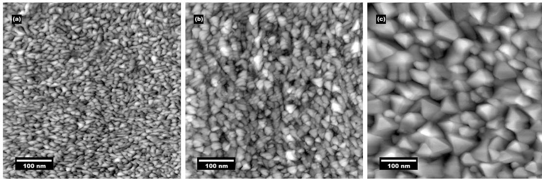
**Figure 5.** STM images of the surface of 85 nm thick Pt films grown on SiO<sub>2</sub> at (a) 27°C, (b) 100°C, and (c) 250°C, respectively.
