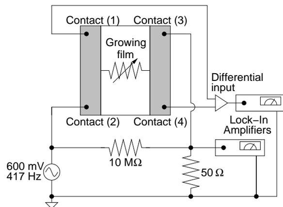
**Figure 2.** The dual lock-in amplifier setup used to measure the electrical resistance of the growing films *in-situ*. The setup is a standard four point probe measurement.
