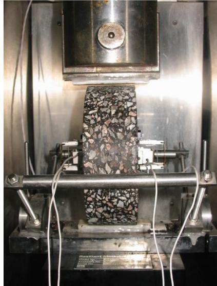
**Figure 2.** The experimental setup of the Superpave IDT test.
