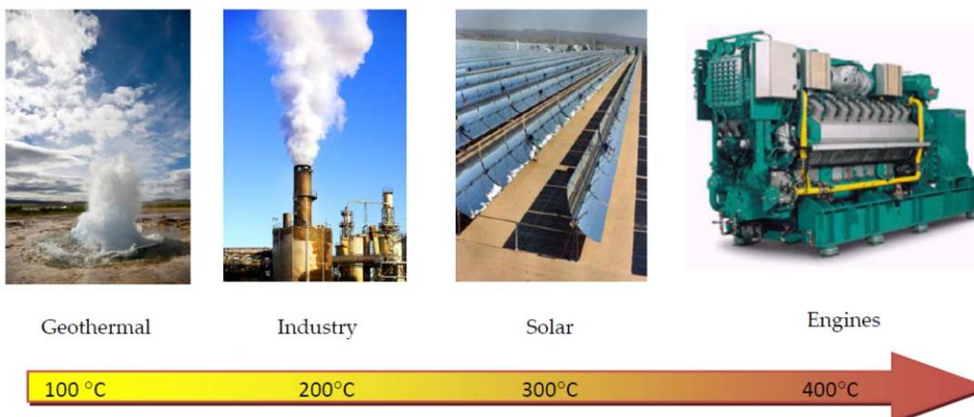
Figure 1 typical temperature range of different heat sources for heat recovery<sup>1</sup>
