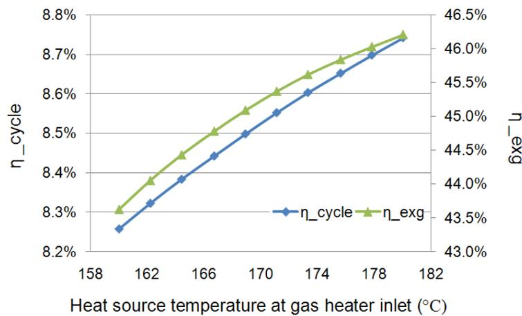
Figure 15 System thermodynamic efficiencies vs. heat source inlet temperature
