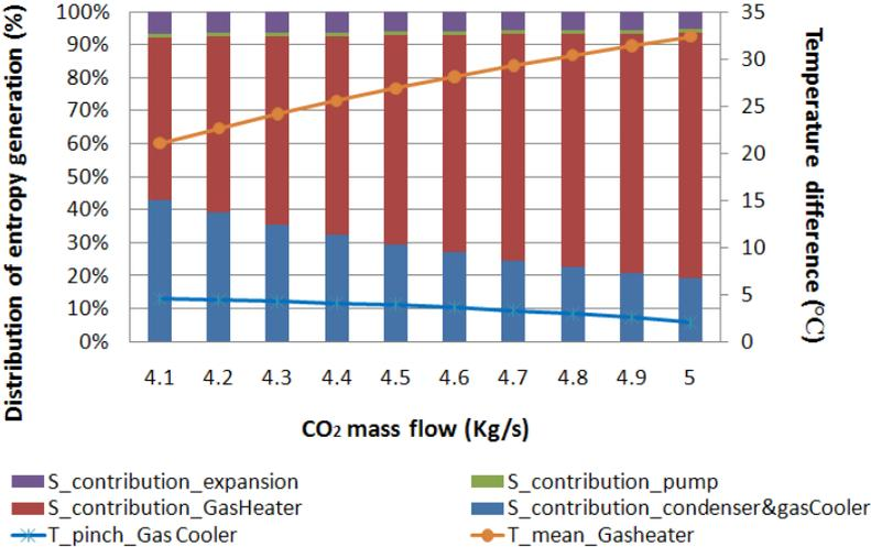
Figure 5 Distribution of entropy generation vs. CO<sub>2</sub> mass flow
