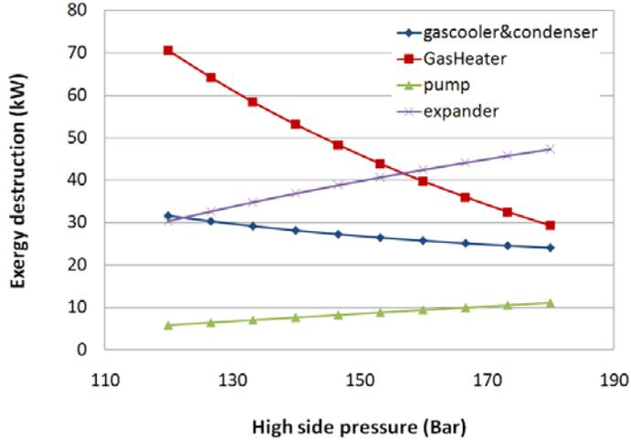
Figure 7 Exergy destruction against system high pressure side pressure
