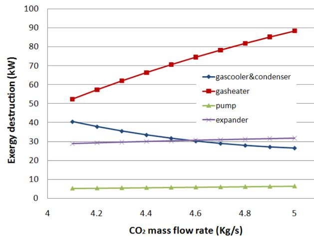
Figure 3 Exergy destruction against CO<sub>2</sub> mass flow rate
