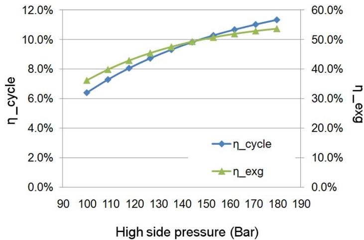
Figure 11 System thermodynamic efficiencies vs. system high pressure side pressure
