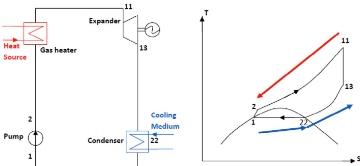
*Figure 2 Schematic layout and the corresponding T-S chart of a CO<sub>2</sub> transcritical power system*
