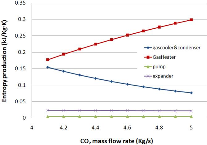
Figure 4 Entropy generation against CO<sub>2</sub> mass flow rate
