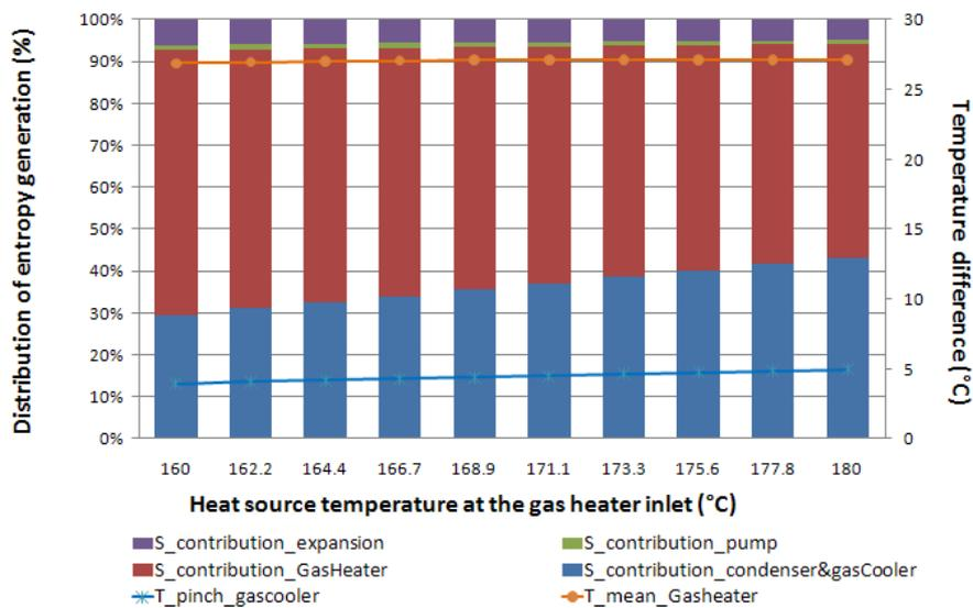
Figure 14 Entropy generation vs. heat source inlet temperature
