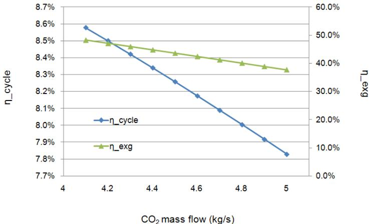
Figure 6 System thermodynamic efficiencies vs. CO<sub>2</sub> mass flow
