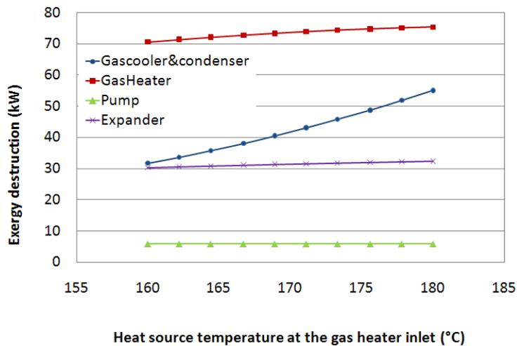
Figure 12 Exergy destruction vs. heat source temperature at the gas heater inlet
