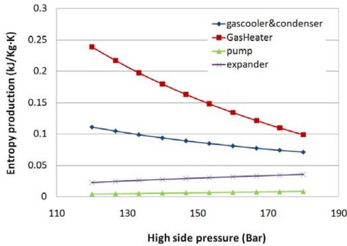
Figure 8 Entropy generation vs. system high pressure side pressure
