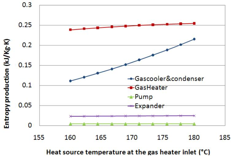
Figure 13 Entropy generation vs. heat source temperature at the gas heater inlet
