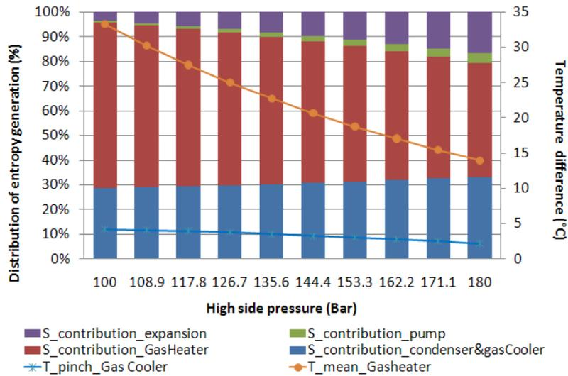
Figure 9 Distribution of entropy generation vs. system high pressure side pressure
