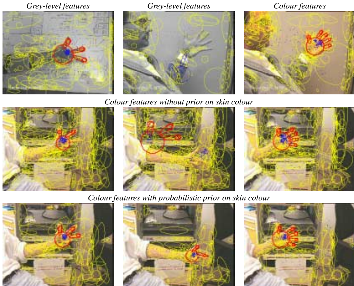
Figure 5. Illustration of the effect of combining shape and colour cues. (First row) (Left) Grey-level features are sufficient for detecting the correct hand pose when there is a clear grey-level contrast between the background and the object. (Middle, Right) When the grey-level contrast is poor, shape cues in colour space are necessary. (Middle row) With no prior on skin colour in cluttered scenes, the system often detects the wrong pose and sometimes also the wrong position. (Second row) When including this skin colour cue, both position and pose are correctly determined.
