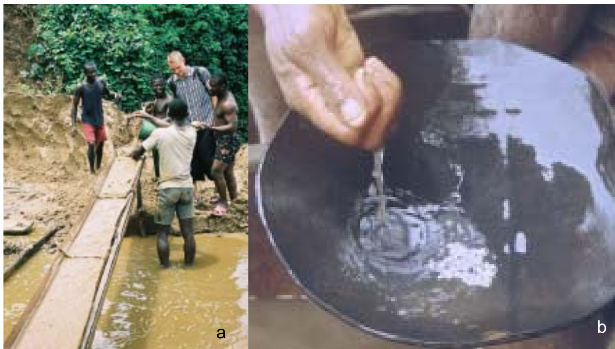
Figure 4. a) Blanket washing of milled ore. The concentrate from this gravity method is repeatedly washed and b) gold amalgam is formed when mercury has been added. (Reproduced after Asklund & Eldval 2005 ).
