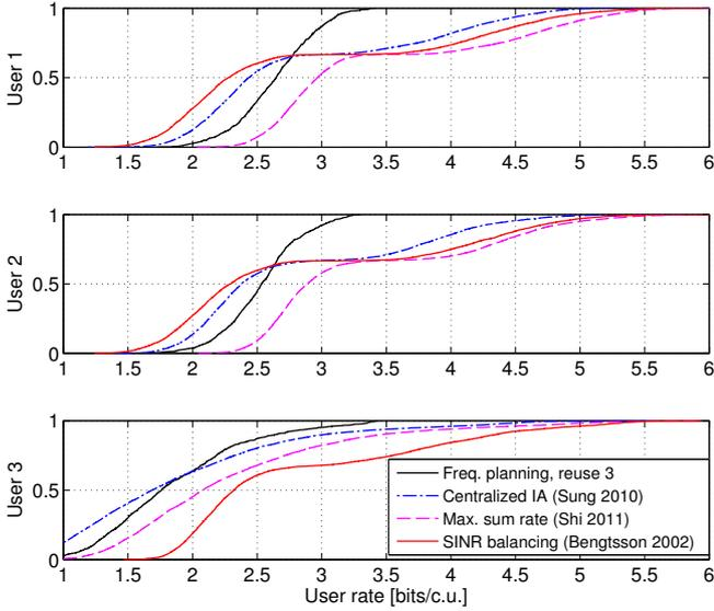
**Fig. 6.** Empirical cumulative distribution function of individual user rates for SNR = 20dB, obtained from 5000 channel realizations.
