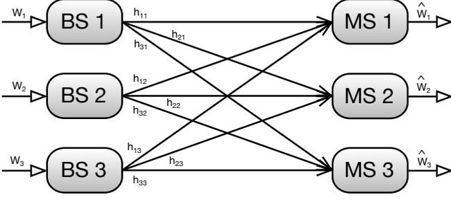
**Fig. 1.** 3-user interference channel with frequency-selective links. Each transmitter transmits a message to its desired receiver, which appears as interference to the other receivers.
