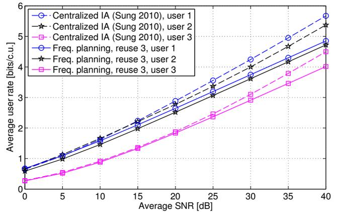
**Fig. 5.** Individual user rates averaged over 500 channel realizations.
