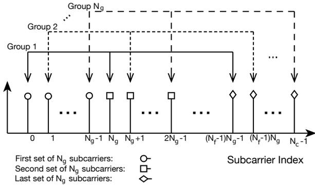
**Fig. 3.** Alignment group structure. Each alignment group contains  $N_f$  subcarriers, and there are  $N_g$  alignment groups.
