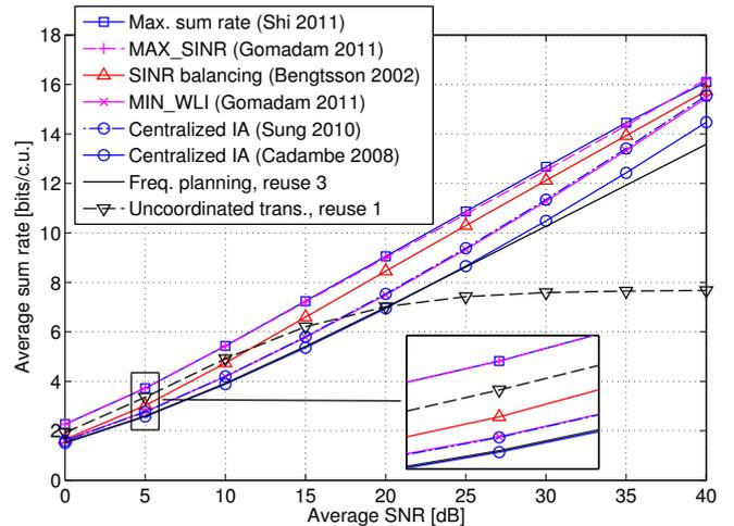
**Fig. 4.** Sum rate averaged over 500 channel realizations.
