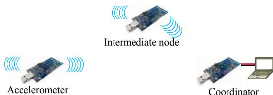
Figure 10. A network scenario with two hops between the sensor node and coordinator.
