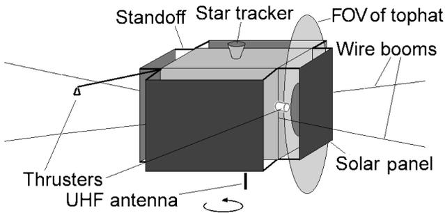
**Figure 1:** Saga configuration. Solar panels are mounted on standoffs and particle sensors mounted behind panels. Wire boom roots are located at the corners. Star tracker is located on the top or bottom platform. UHF antenna for communication to mothership is located on the top and/or bottom platform. Cold-gas or propane thruster is located on the short boom to make the thrust vector parallel to spin vector.
