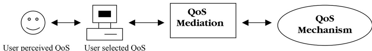
**Figure 18: Model of the QoS provisioning chain**
